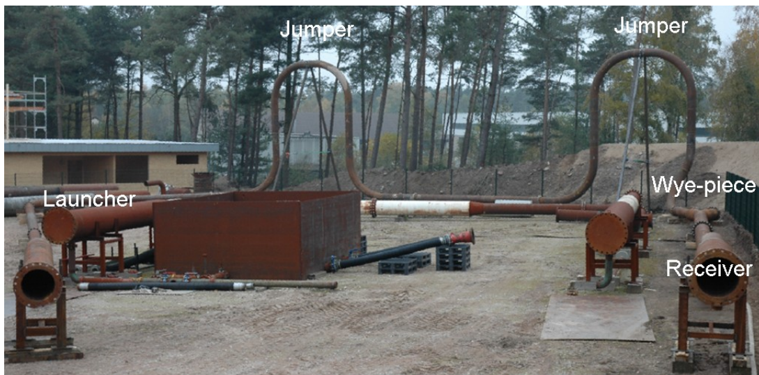
Figure 6: The 14"/18" test loop
