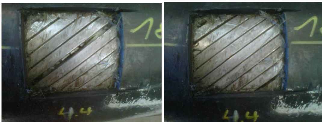
Figure 4: Rearranging layers allows introducing small defects into inner layers.
