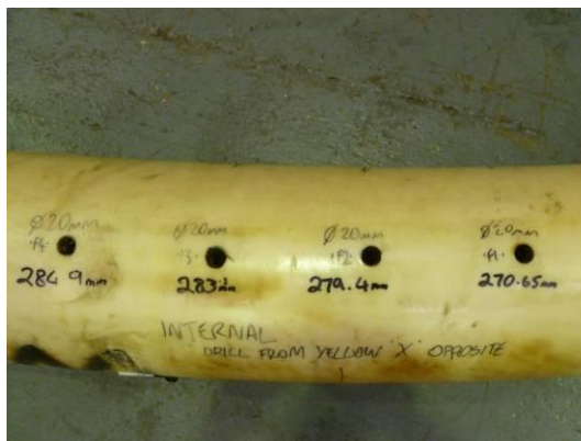
Figure 3: Obtaining internal metal loss defects by drilling holes from the opposite side into the inner layer.
