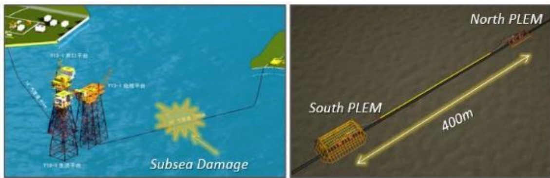
Figure 1: Anchor damage location
