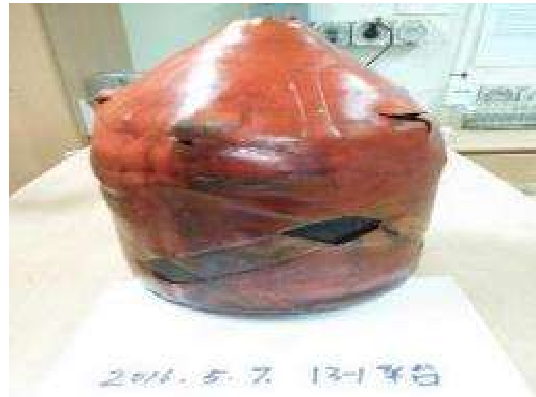
Client routine pig at receive
