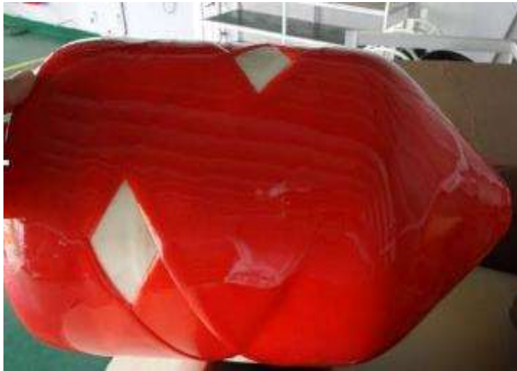
Client routine pig prior to launch
