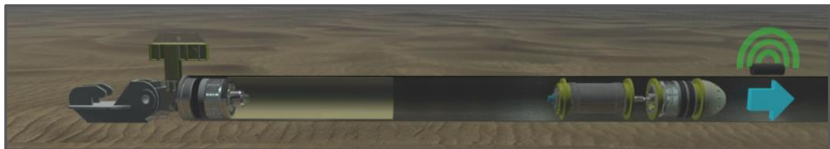
PRT set in pipe end and Tecno Plug pigged into pipeline for dewatering
