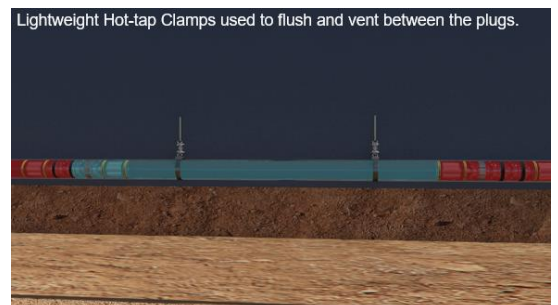
8. Small hot taps for venting and flushing
