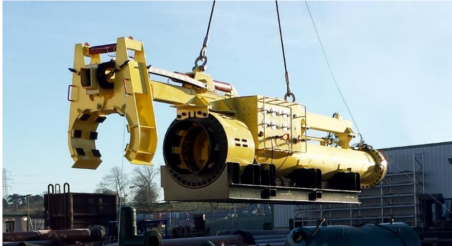
Subsea Diverless Flangeless Launcher
