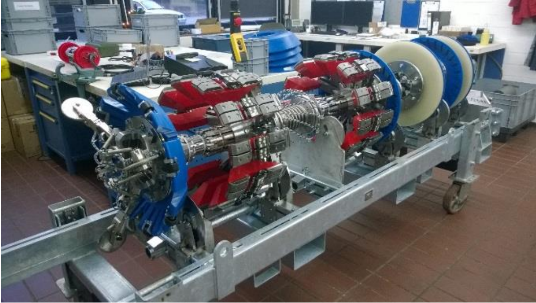
Figure 4 Combo magnetizer optimized for negotiating ID range, wax as well as for full measurement performance in the PL120 pipeline
