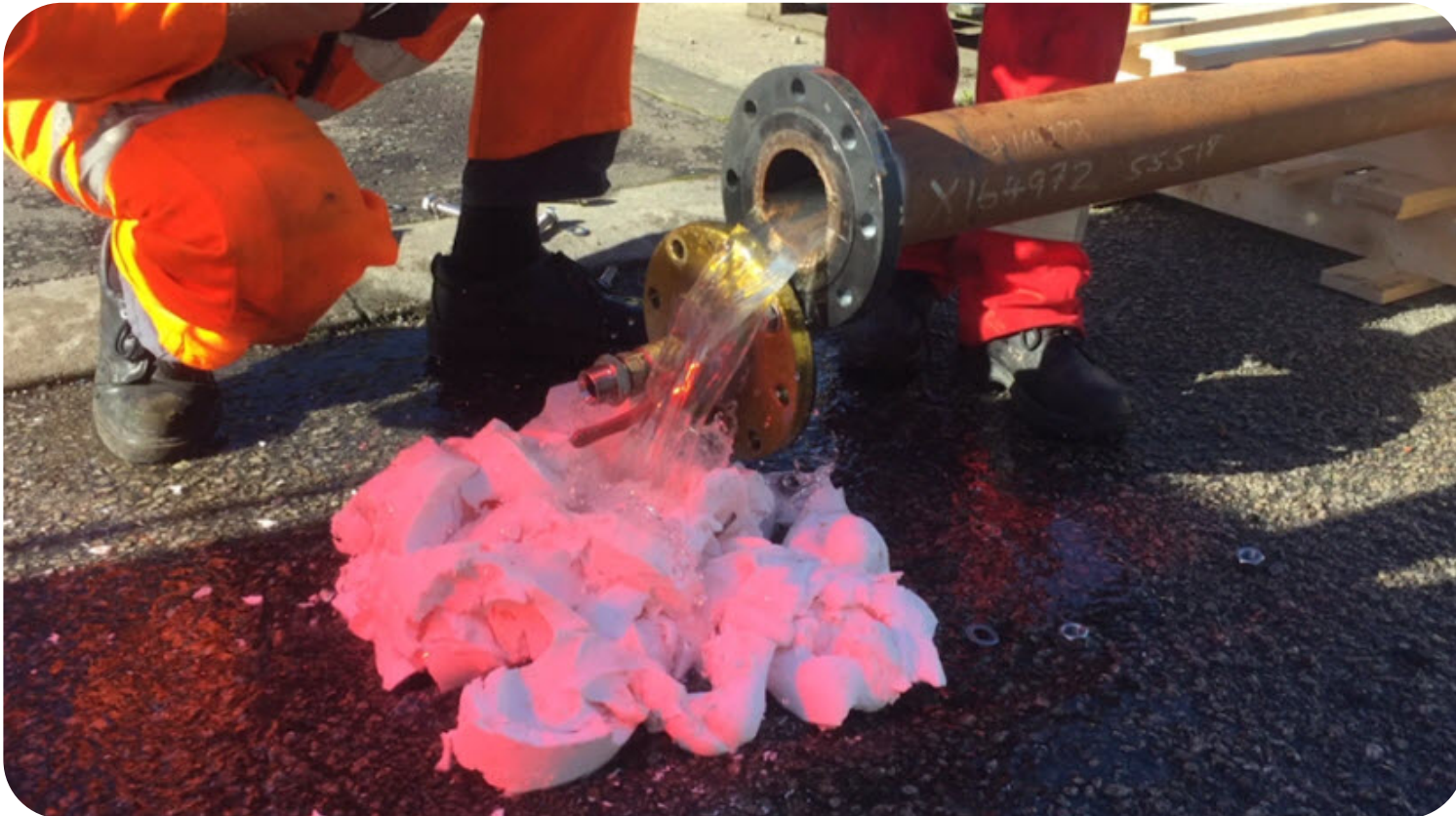
4" EVO-PIG plug was extruded 100% throughout 1" valve
