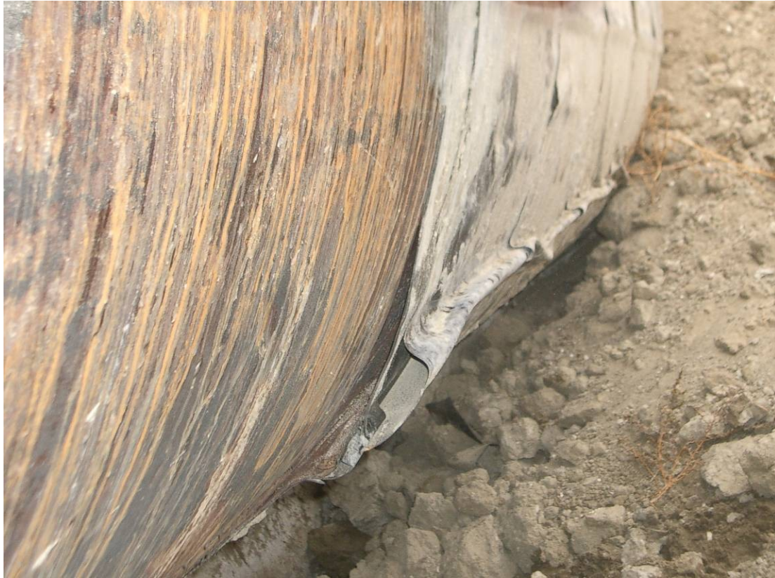
Figure 8 Rucking of a Tape Coating
