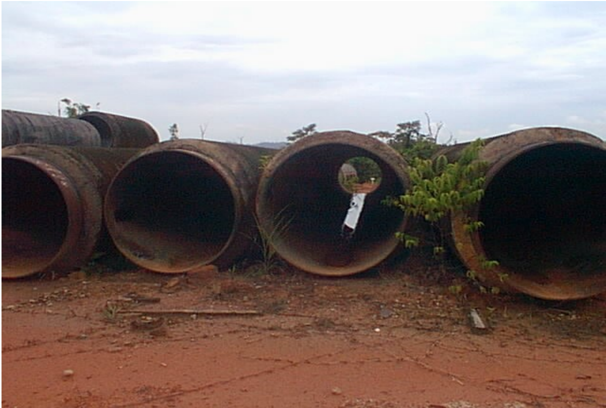
Figure 3 Pipe in Storage With Surface Internal Corrosion
