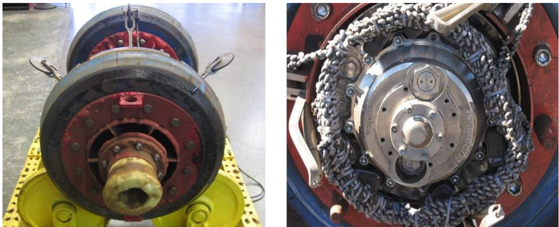
Figure 6 – Post-run Images of EGP tool (left) and MFL Tool (right)
