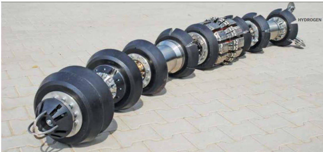
Figure 4 – ATEX Compliant MFL ILI Tool
