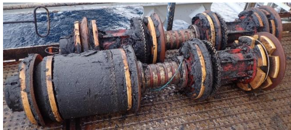
Figure 2. Illustration of operational cleaning pig and photo of cleaning pig after pig run.
