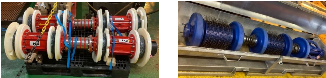
Figure 5. Pictures of Reinhart Tiger tool and swabbing pigs
