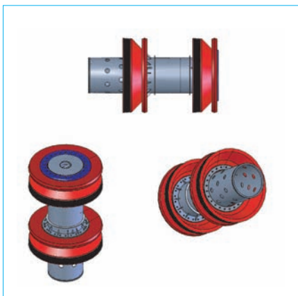
Modified pigs used for the batch launcher.
