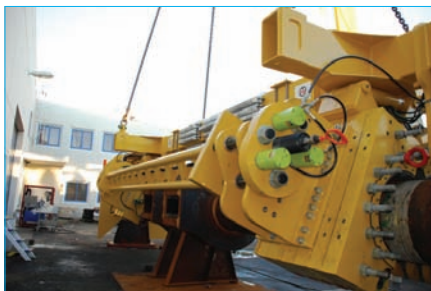
The Kvitbjorn clamp positioned on a pipeline identical to Kvitbjorn pipeline.
