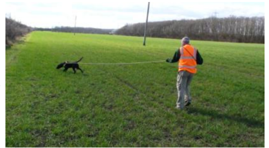
Trained dogs deployed as leak detection tool.
