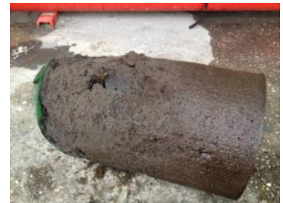
Anode Retaining Strap Embedded in Foam Body
