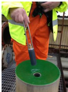
Loading Caliper Cartridge and Transmitter
