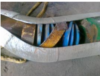
Bi-Di Pig with Dislodged Anodes
