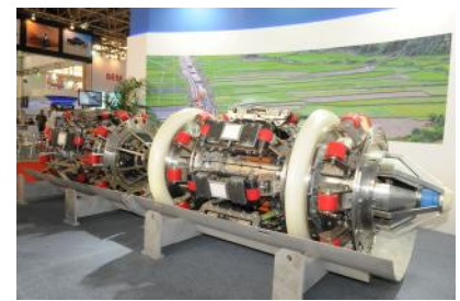
CPPI's 48inch EMAT Crack Inspection Pig
