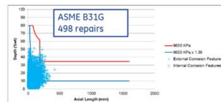
Distribution of external metal loss according to depth and distance along pipeline
