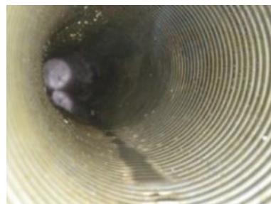
Fig. 3: Dewatering test of EVO-Pig in rough bore flexible riser
