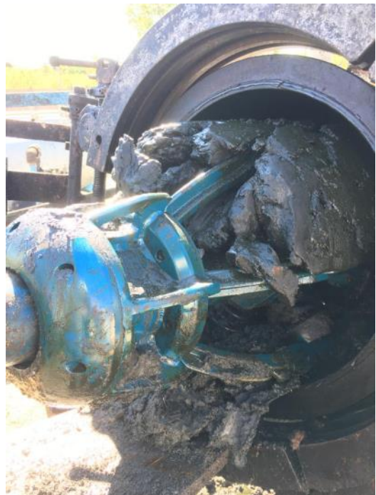
Wax debris removal
