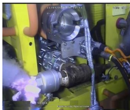
Fig. 4: ROV Footage from successful dewatering showing pig extrusion
