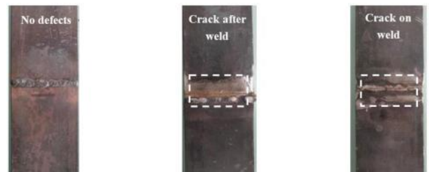
Figure 9. Physical image of experimental welded steel bar
