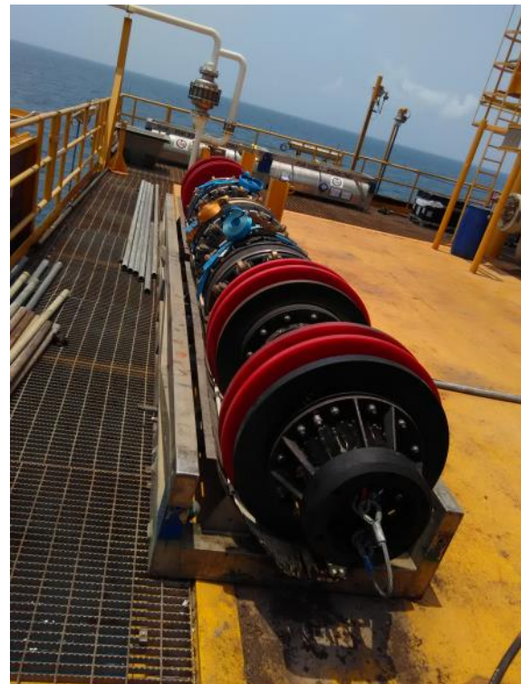
A 3-module, 32-inch SmartPlug® tool ready for launch on an offshore platform
