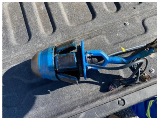
i2i's 4inch NMP Pioneer tool after an inspection run in 1.4km of flexpipe
