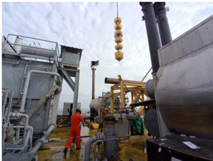
Morken Group's MFL HR tool with Introscope® module
