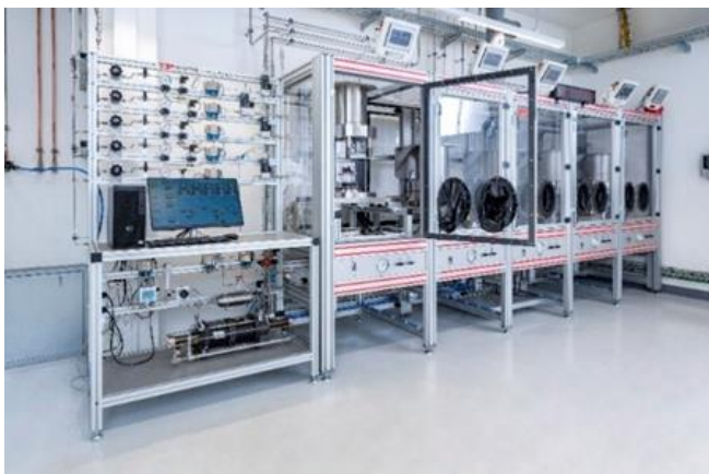
ROSEN's hydrogen laboratory is equipped with 5 autoclaves connected with an automatic gas mixing unit.
