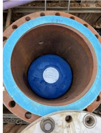
Foam pig with transmitter cavity
