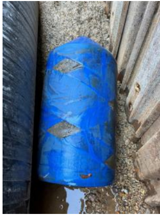
Undamaged pig post run (2 nd visit)
