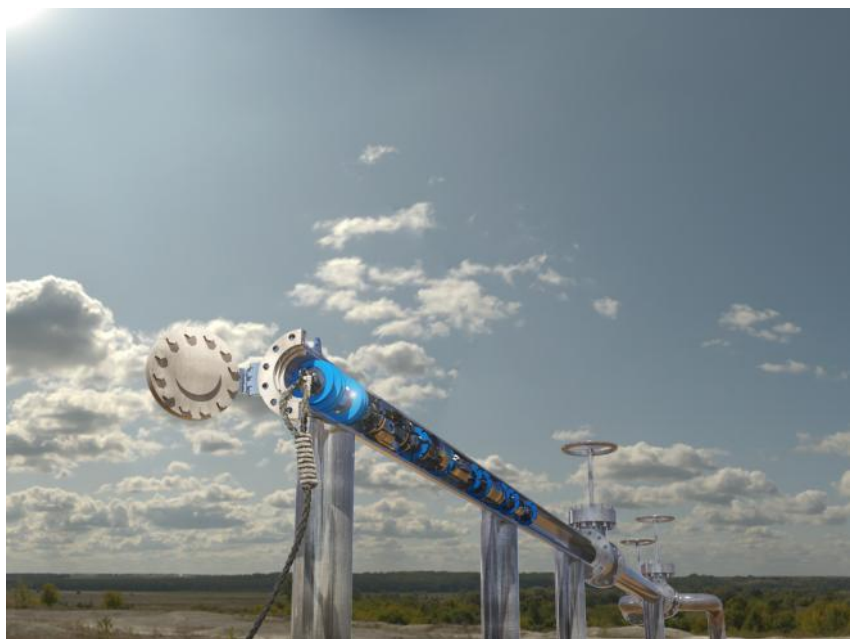
Pipecare Group Inline inspection using a tethered UTWM Crawler
