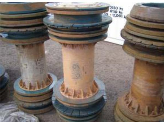
Figure 5: Condition of pigs after dewatering completed
