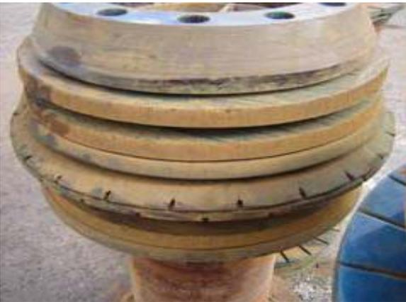
Figure 4: Condition of pigs after dewatering completed
