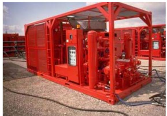
Figure 2: Main compressor unit
