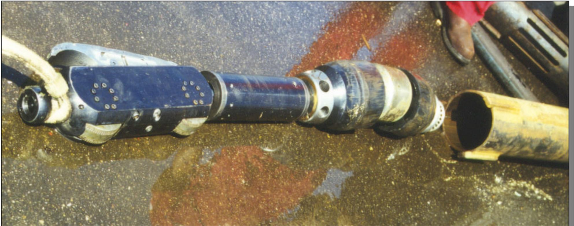
HAPP™ after a cleaning run of the 7.3 miles, 6.25 inches Braheney Line [operated by Equilon Pipeline Company, Denver City, TX pipeline contained 4 elbows à 22.5°, radius: 1.5 D]
