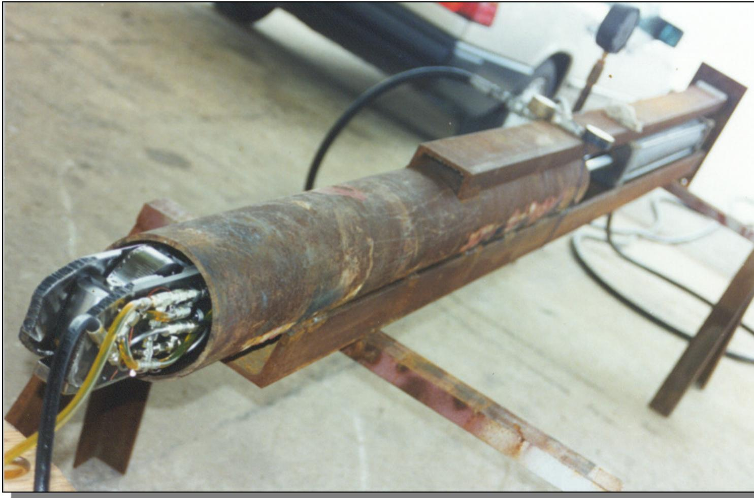
Test set-up to determine the brake systems' travel speed/brake force characteristics. A hydraulic ram was used to pull the brake systems through a pipe section.
