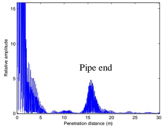
**Figure 3** Matched filtering analysis of the reflections of 800Hz waves
