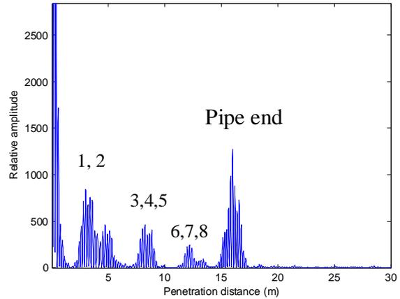
**Figure 6** Matched filtering analysis of the reflections of the chirp signal
