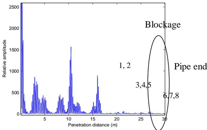
**Figure 7** Blockage detection using chirp signal
