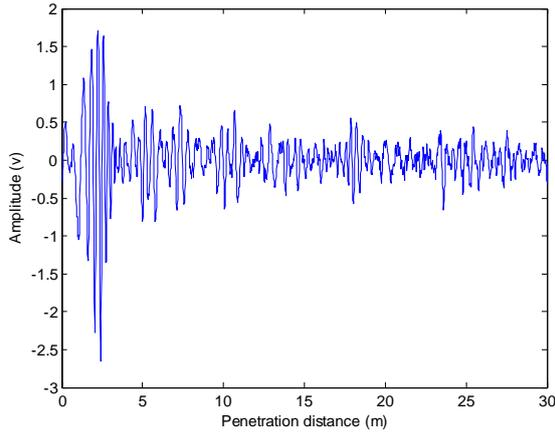
**Figure 5** Reflections of 0-800Hz chirp signal
