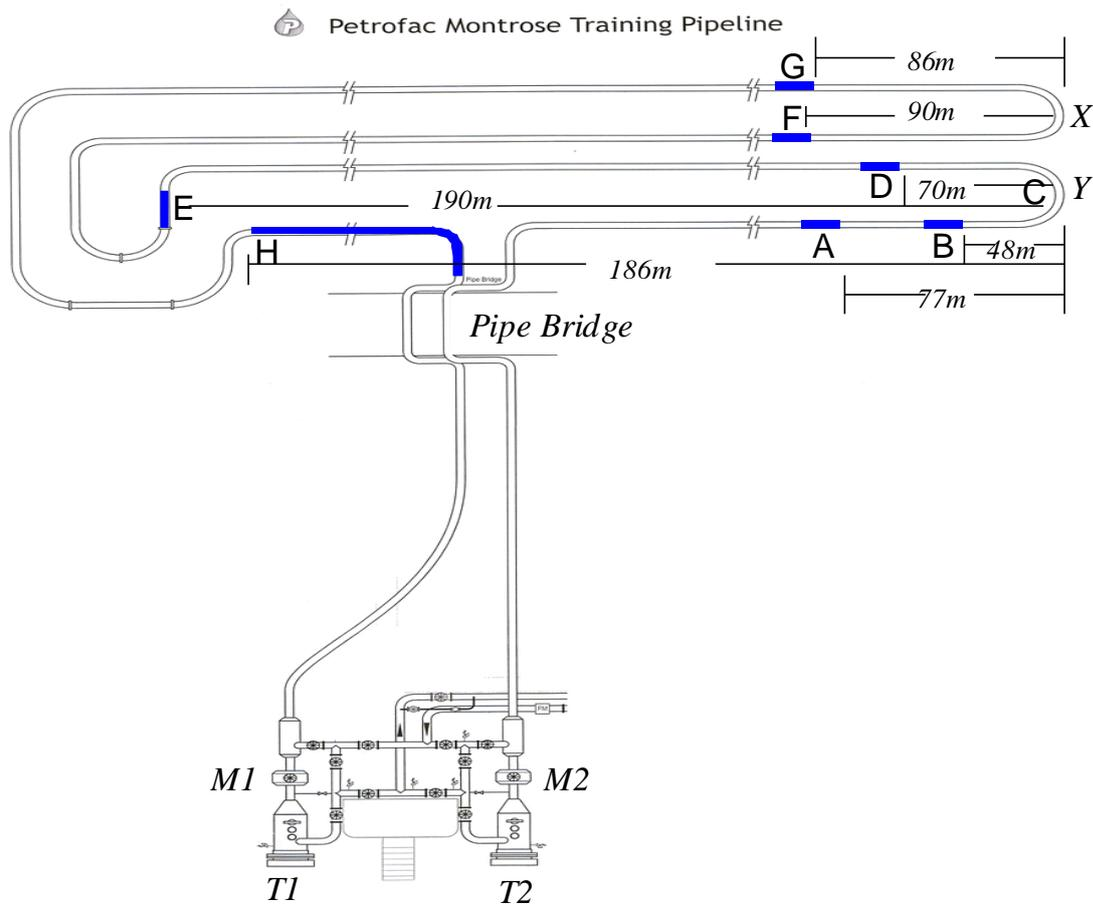
**Figure 9:** Location of the blockage features identified located in the pipeline
