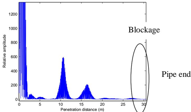
**Figure 4** Detection of a blockage in the pipe
