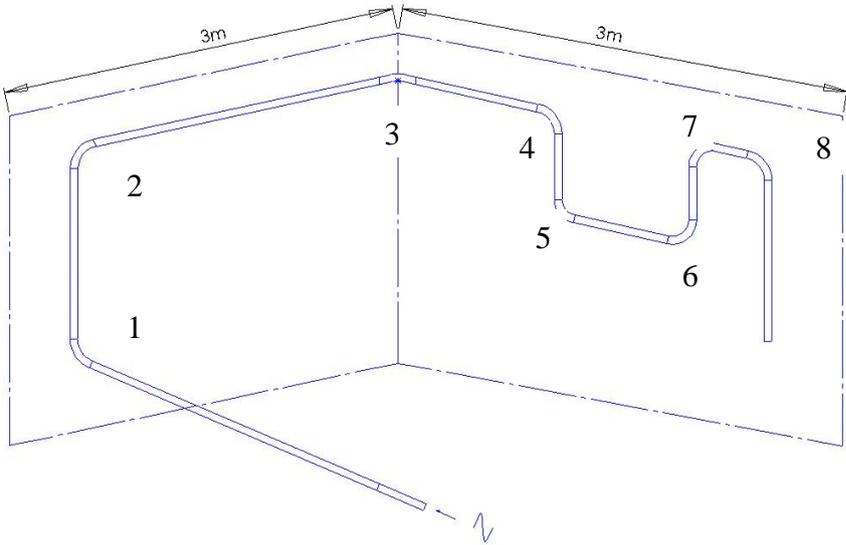
**Figure 1** Schematic of 16m rigid PVC pipe
