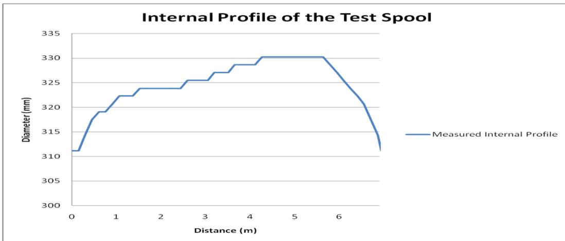
**Figure 8 Measured Internal Diameter of the Defect Piece**
