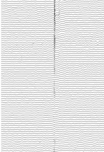
**Figure 1 Showing the weld signal virtually disappear completely at some clock positions.**
