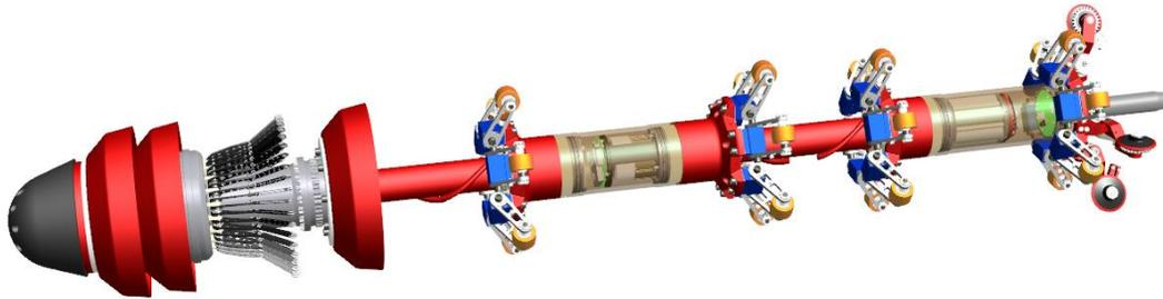
**Figure 3 Schematic of the 12" High resolution Geopig Tool**
