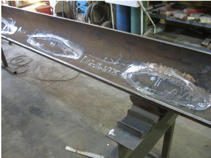
**Figure 4 Showing Defects welded back into Pipe Sample**
