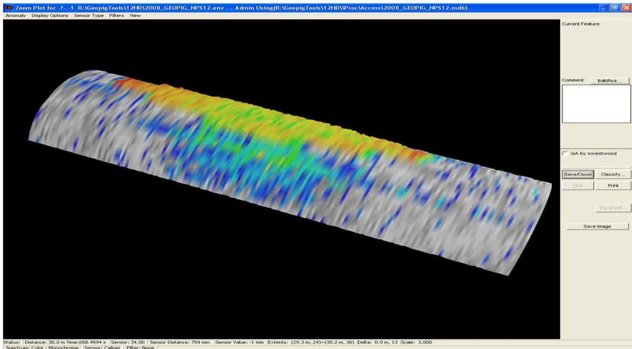
**Figure 7 Sensor Response from the 4.7mm Deep Defect**
