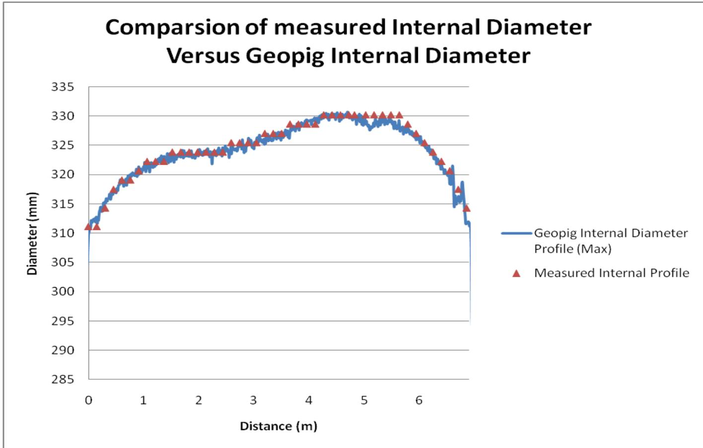
**Figure 11 Comparison of the maximum measured internal diameter from the Geopig with the manually measured internal diameter**
