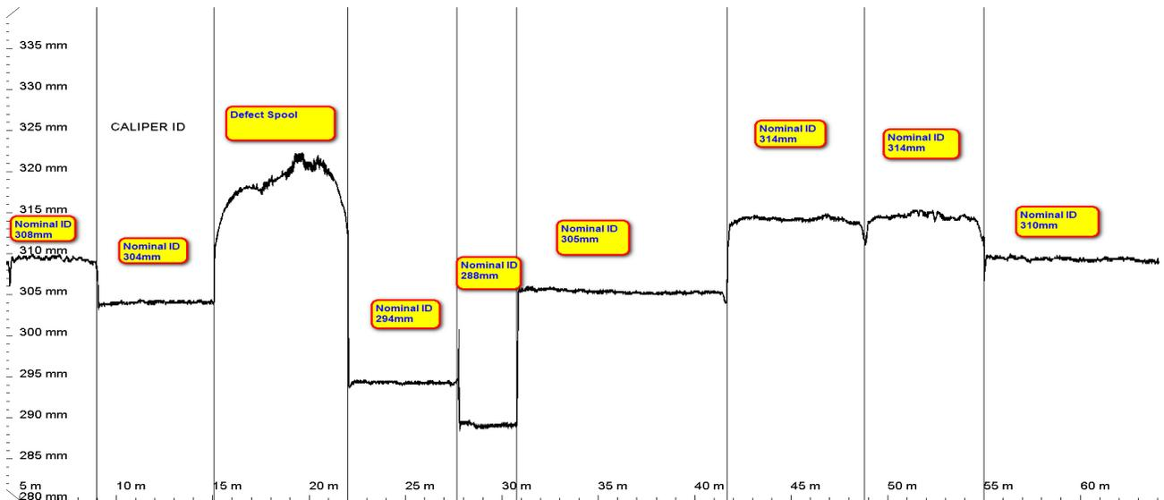
**Figure 10 Comparison of Internal Diameter**
