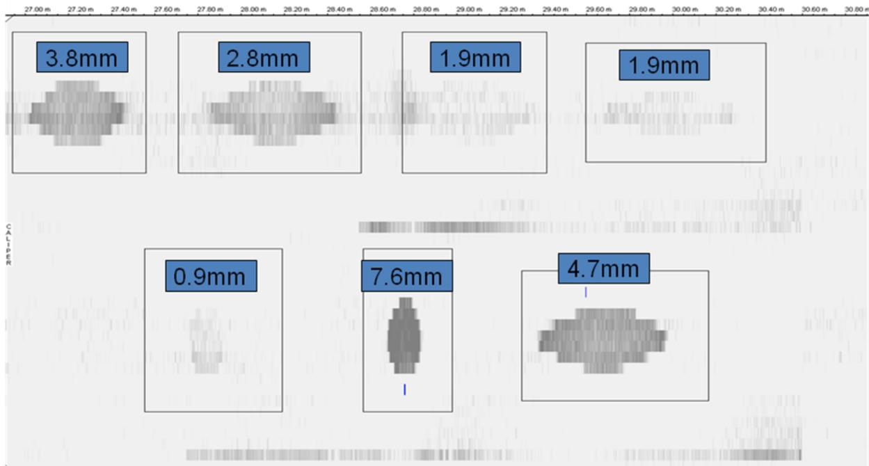
Figure 5 Showing the sensor response for the defect spool.
