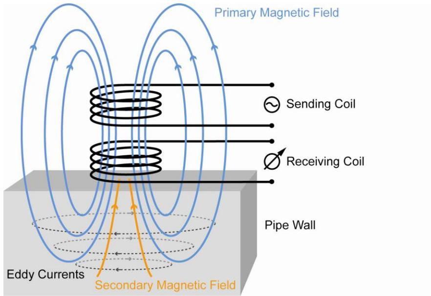
Figure 2: Schematic sketch of coil system for measuring metal loss.
