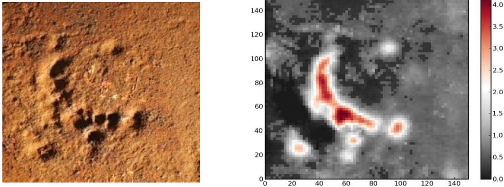
Figure 5: (*left*) Pitting corrosion in a steel plate. (*right*) The corresponding data made with a SIC sensor in a laboratory setup with sample spacing of 2 mm in both directions and a specific pseudo-lift-off scaling (all values in mm).
