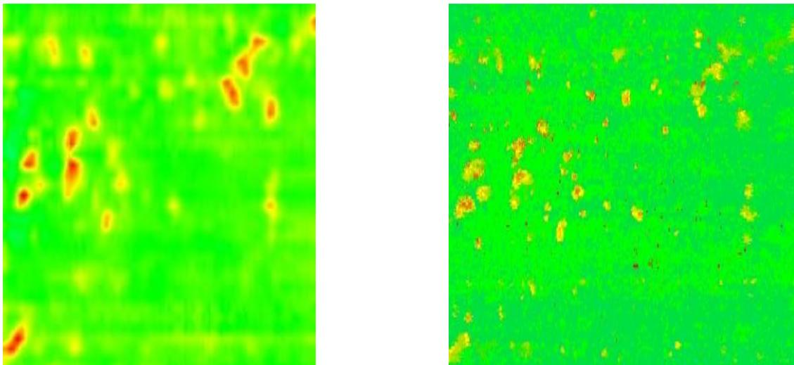
Figure 6: Top of line corrosion in a test pipeline. The left panel shows inspection results obtained with a SIC tool, the right figure represents data derived from an automatic UT measurement. Corrosion patterns in both excerpts can easily be correlated.
