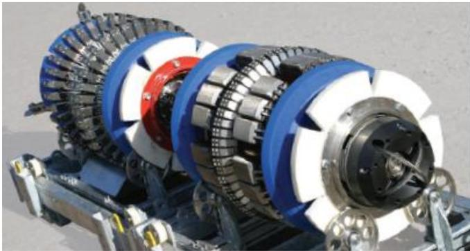
Figure 1: Combination of inspection technologies on a single 30" ILI tool. The front unit consist of a high-resolution MFL unit, the second unit is utilizing a combination of high-resolution geometry sensor with SIC probes.
