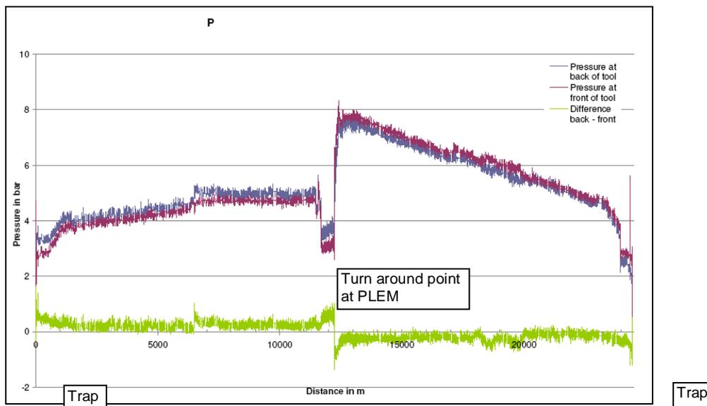
Fig. 7: Pressure recording during MFL run by the inspection pig
