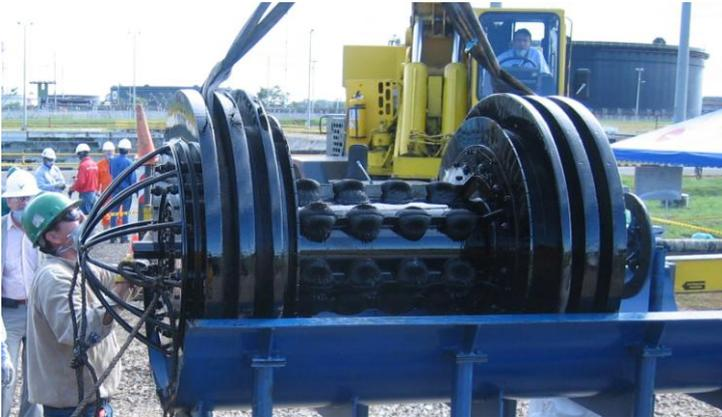
Fig. 3: Cleaning pig equipped with gauge plates, transmitter, magnets and inertial system after the run
