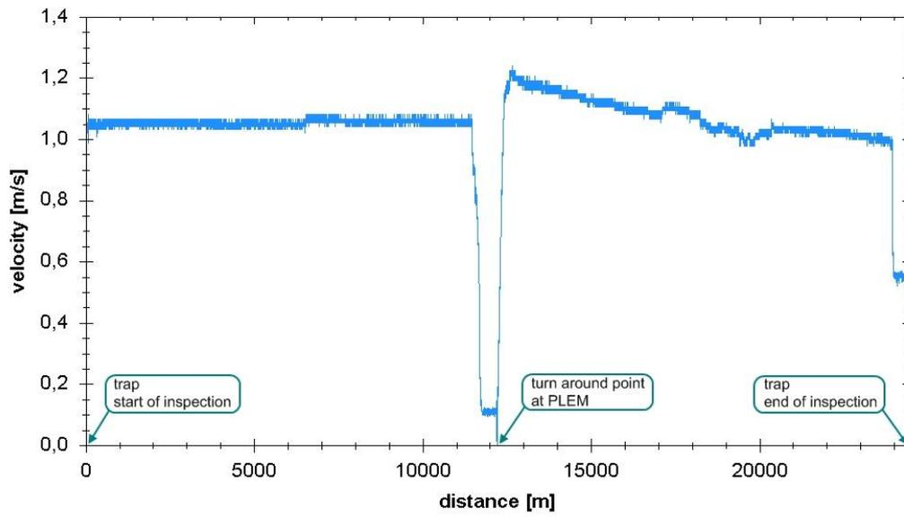
Fig. 8: Speed profile MFL run, top shore to PLEM, bottom PLEM to shore
