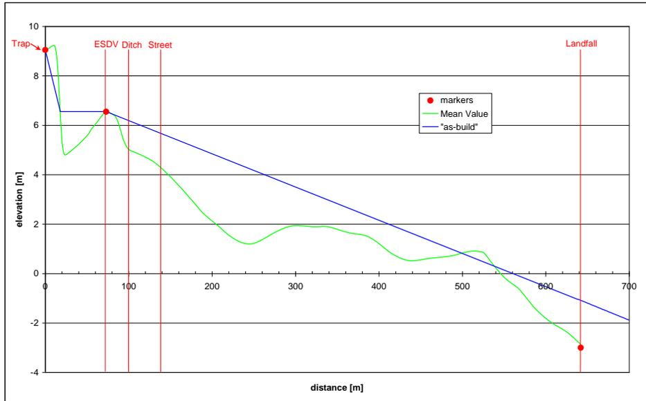
Fig. 6: Vertical pipeline profile onshore section
