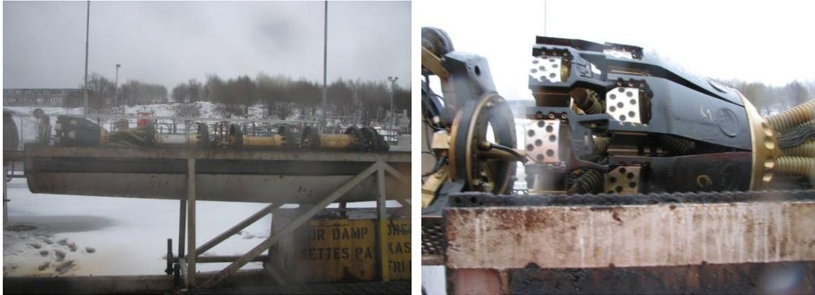
*Receipt of clean 16" Ultrasound- based ILI after successful inspection of TOR1 pipeline at Mongstad*
