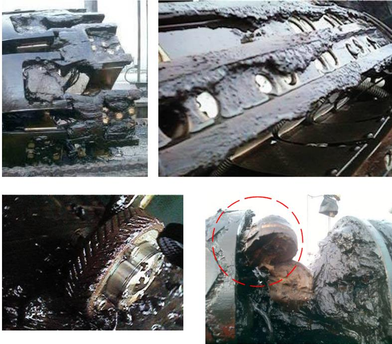
*Example of wax covered sensor carriers on top and odometer wheel on bottom.*
