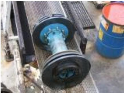
*Disc Type pig with gauge plate*
