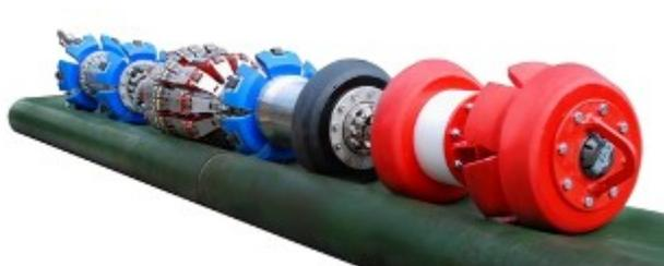
**Figure 3: 12" intelligent in-line inspection tool configured specifically for low flow / low pressure pipelines. To minimize friction for a smooth run performance, non-magnetic rollers (mounted on the blue cups) are used.**
