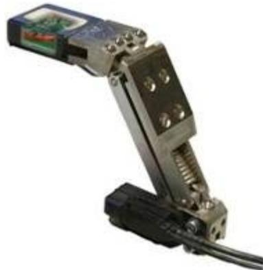
**Figure 7: The mechatronic solution: a touchless electronic sensor is integrated inside the sensor head and a position sensor attached at the bottom monitors the mechanical position of the sensor arm.**
