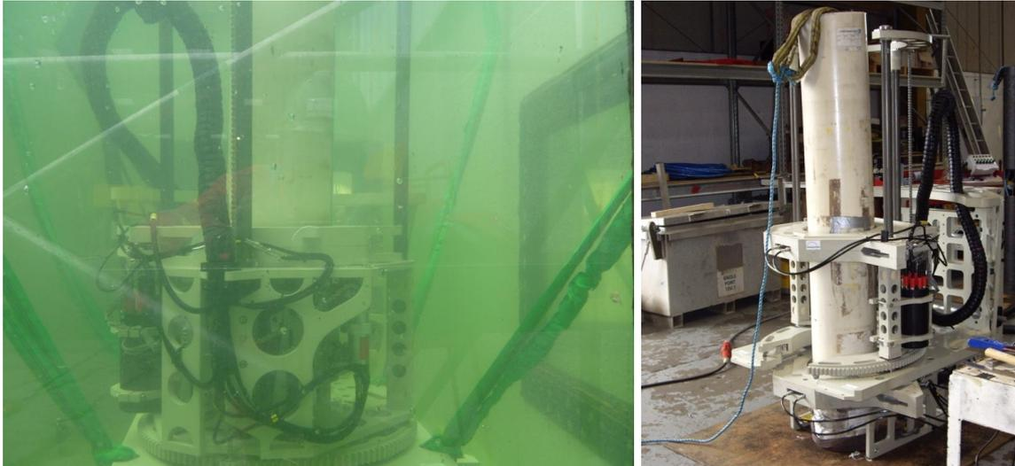
**Figure 6: Newly built inspection tool for flexible risers**
