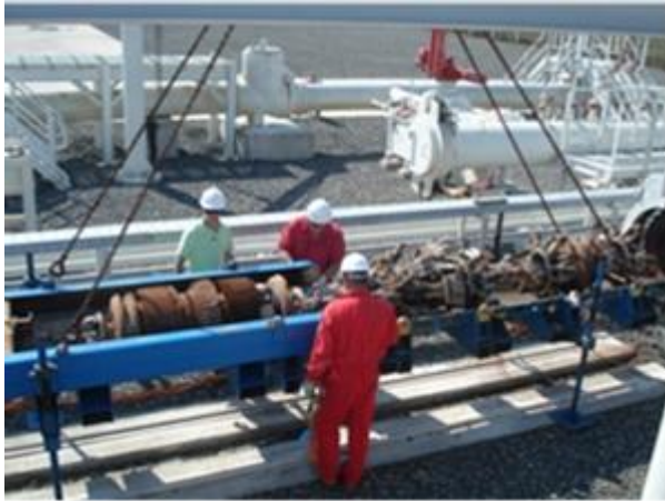
Figure 10 -The MFL pig received in Turkey after 387Km run
