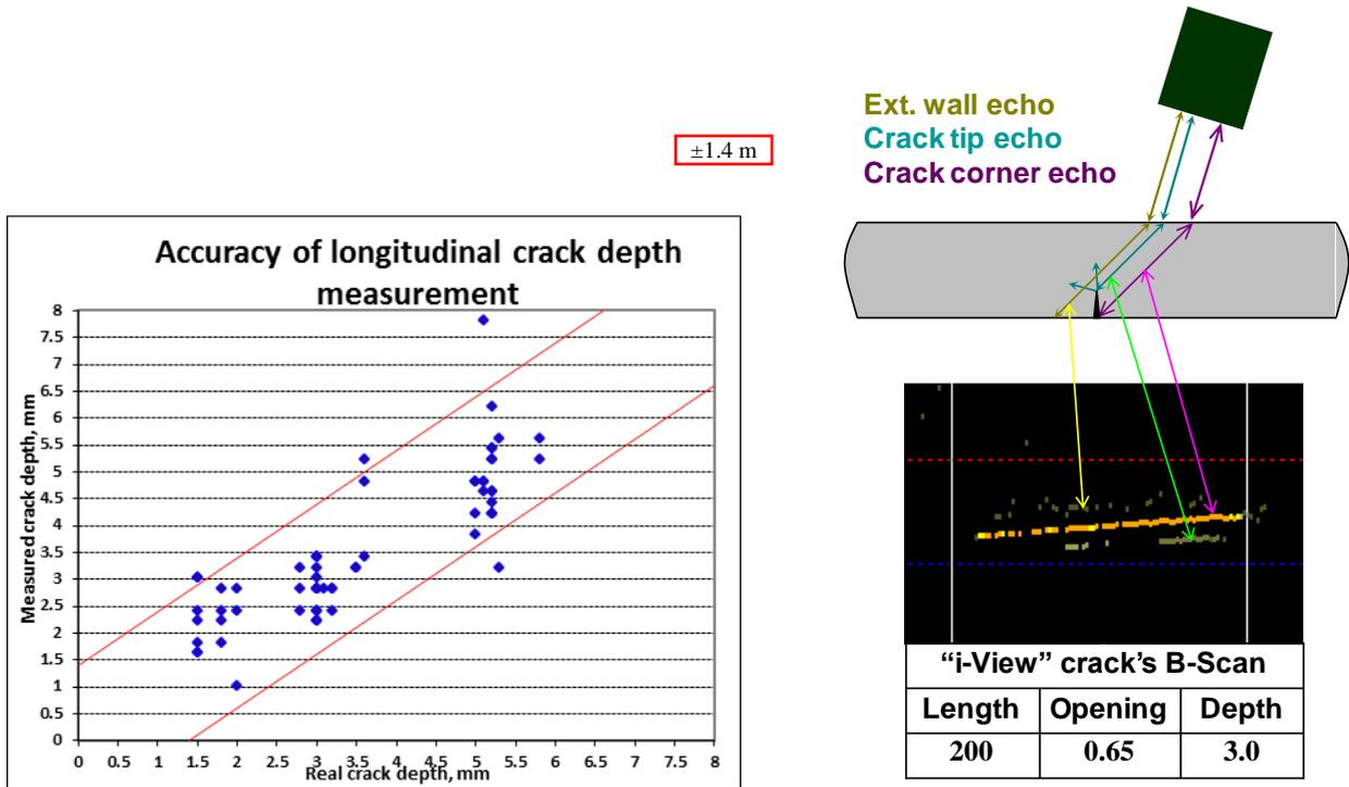
**Figure 6 – Sizing accuracy tests based on echoes' time evaluation (illustration on the right)**
