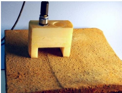
**Figure 4 – Sensor lab test for surface roughness capability**
