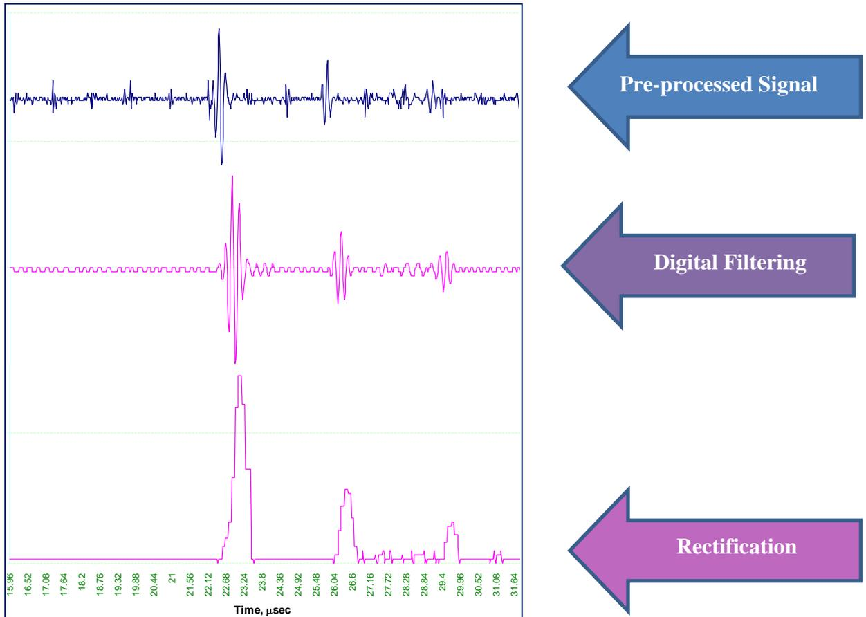
**Figure 3 – Illustration of noisy weak echo signals with onboard digital filtering process followed by rectification process for improved detection and recording accuracy**
