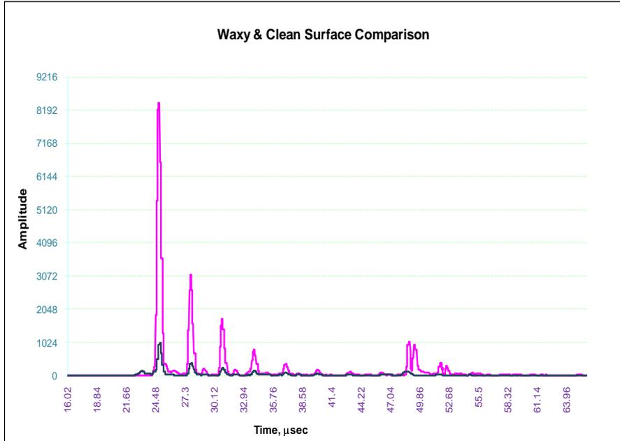
Figure 7 – WM sensor echoes comparison: 1mm hard wax deposit (blue) and clean internal surface (magenta)
