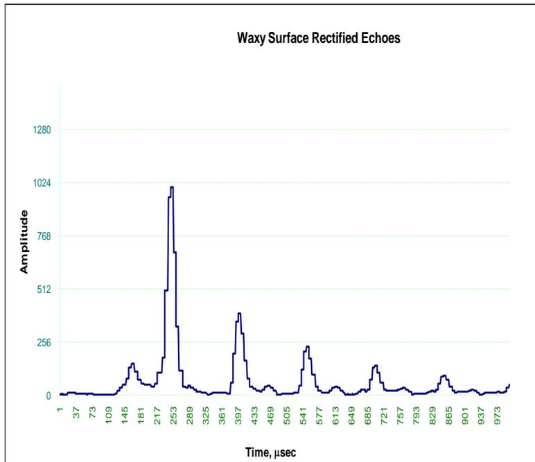
Figure 8 – WM echoes with 1 mm hard wax deposit (zoomed), measurement capability is maintained
