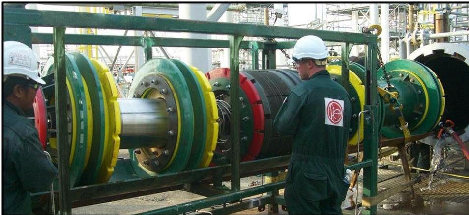
**Fig 8: 38" Tecno Plug™ Deployment Malaysia**
