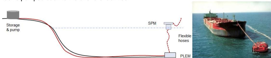
Figure 6: Schematic layout of a typical loading line (left) / Tanker connected to a monobuoy (right)
