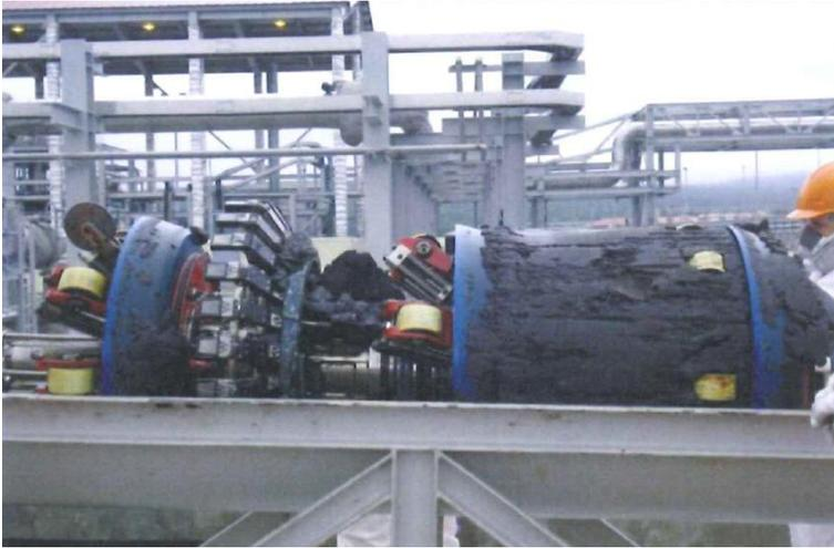
**Figure 4: MFL/Geo tool after run in insufficiently cleaned pipeline**
