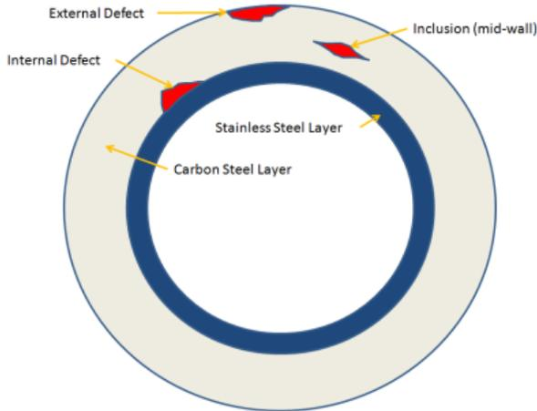
**Figure 5: CRA Pipeline with defects**
