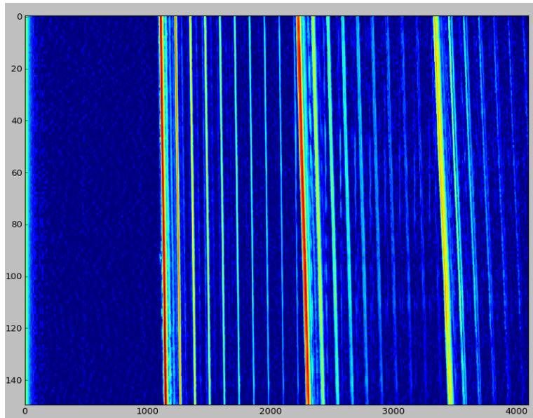
**Figure 29: UT data for 16in pipe spool**
