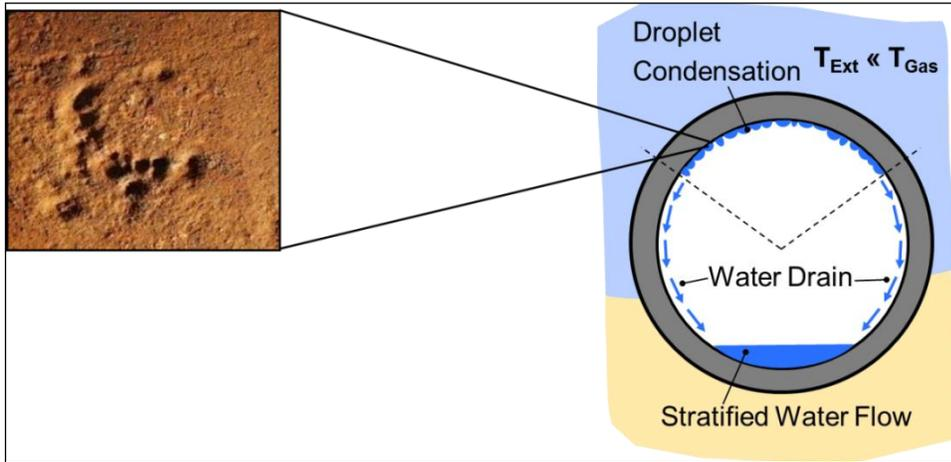
Figure 1: Top of line corrosion
