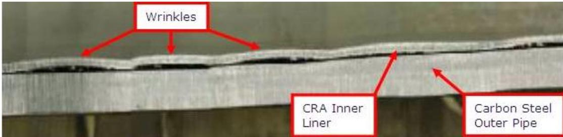
**Figure 6: CRA Pipeline with defects (2)**
