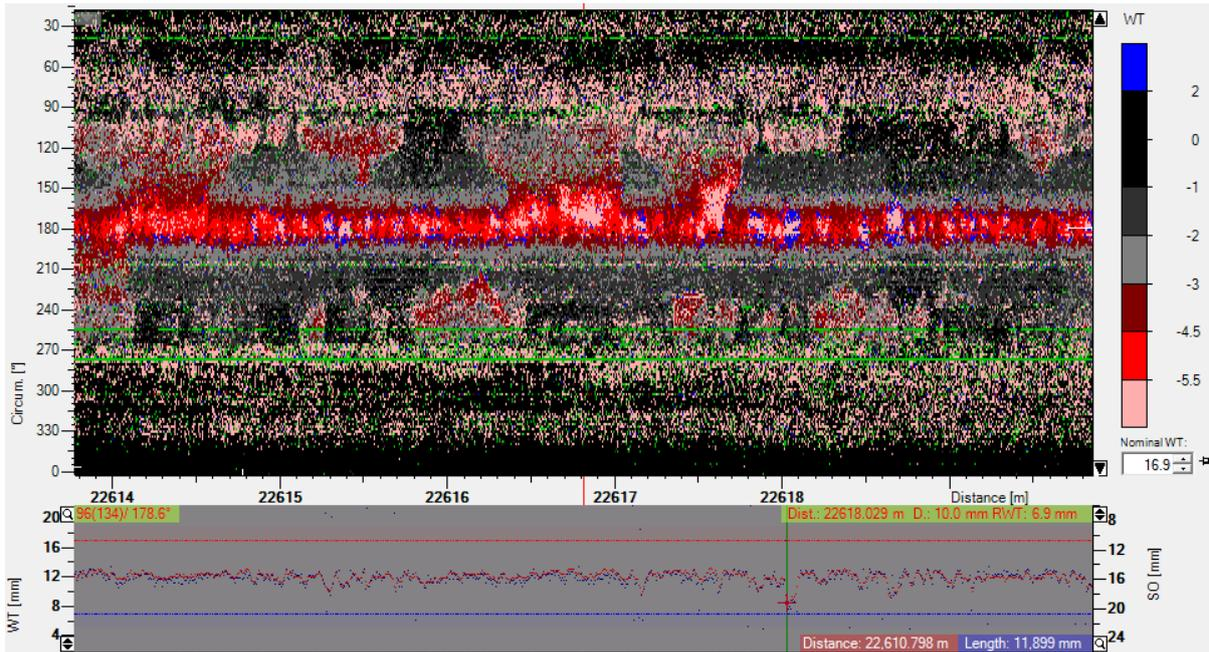
**Figure 2: Long axial corrosion with a complex and rugged shape**
