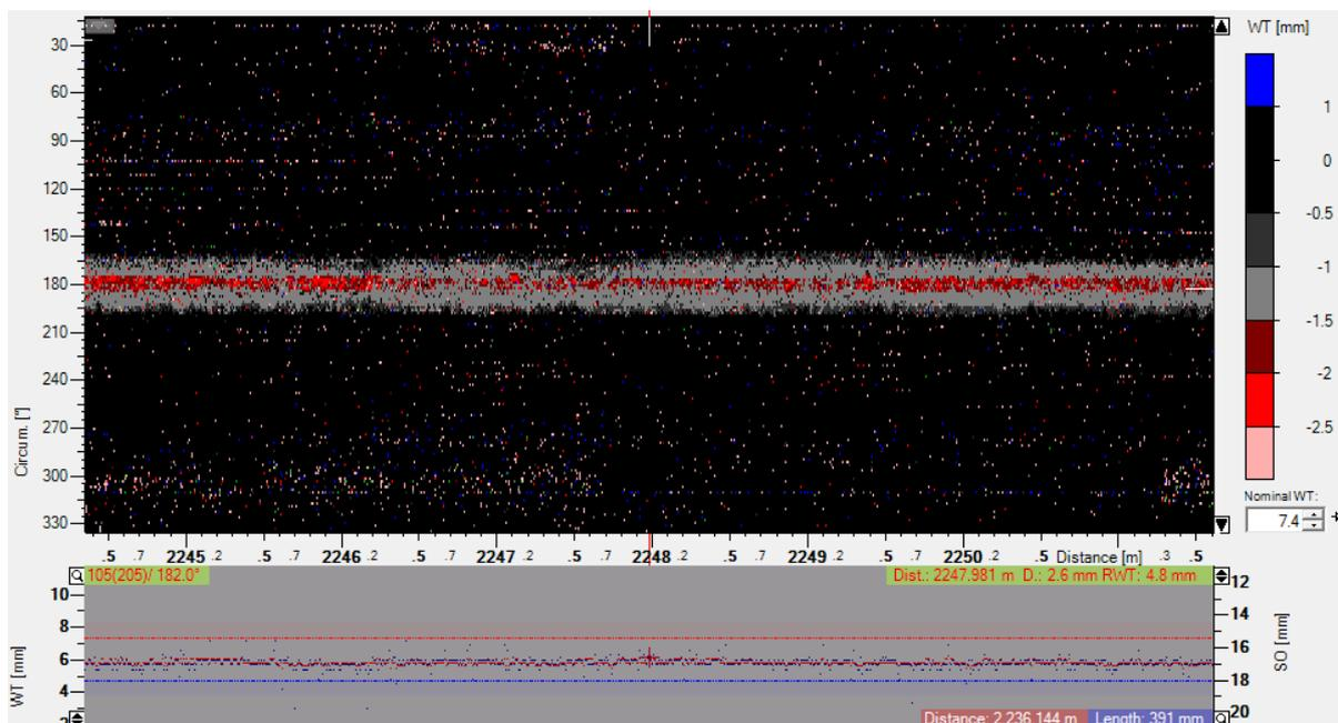
Figure 1: Long axial corrosion with a smooth and even shape
