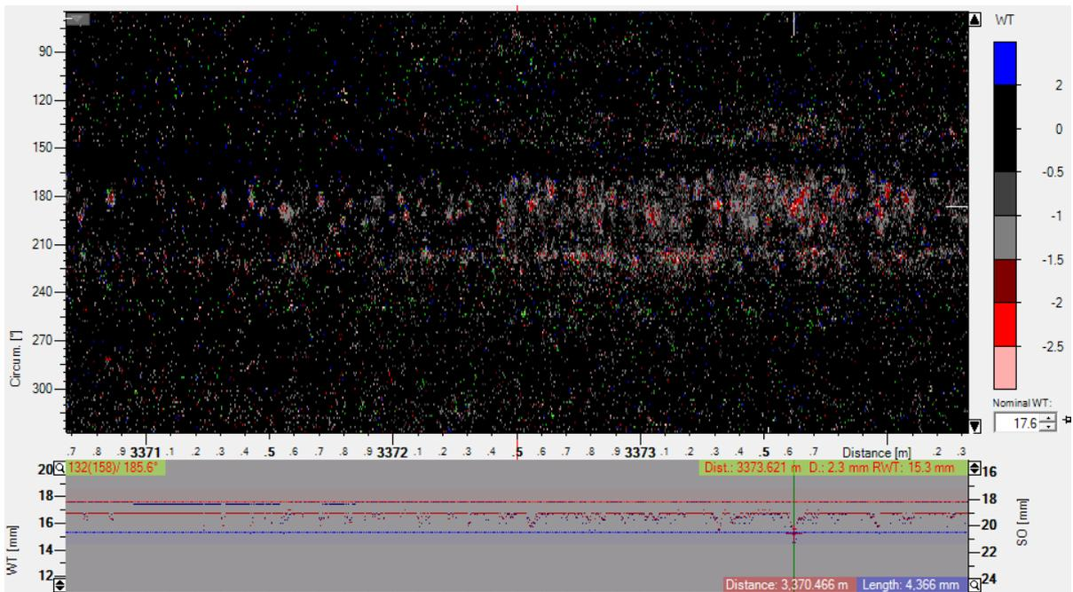
**Figure 3: Chain of pit-like corrosion spots along the 6 o'clock position**
