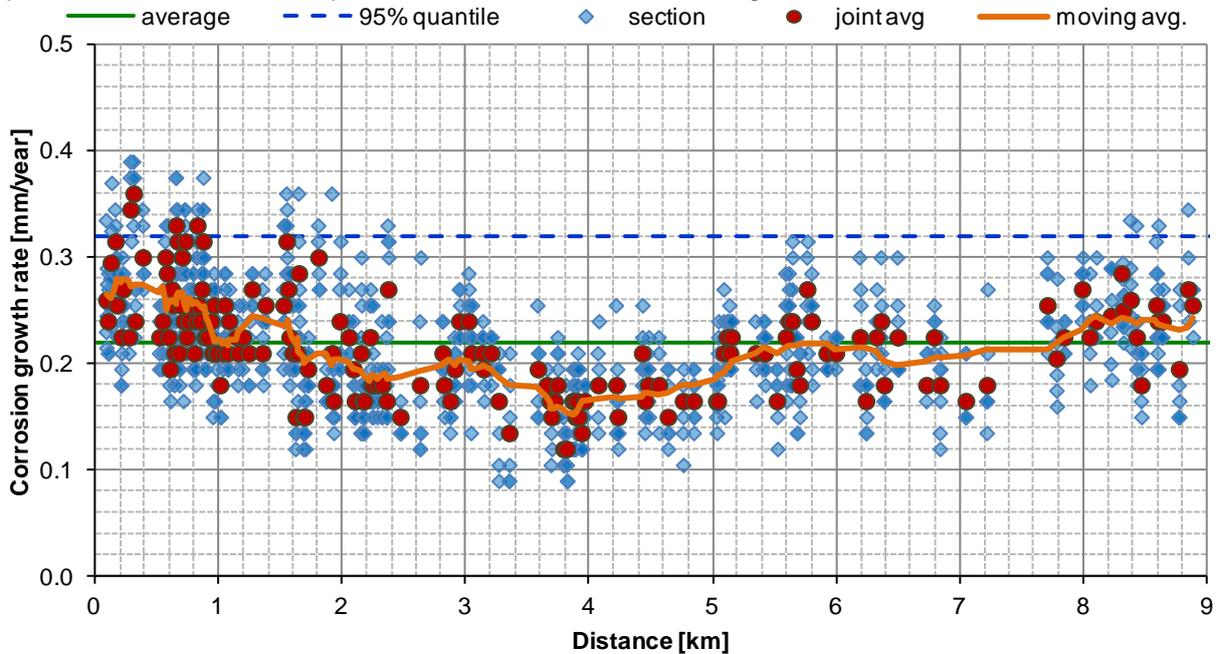
Figure 11: Corrosion growth rates versus distance along the pipeline
