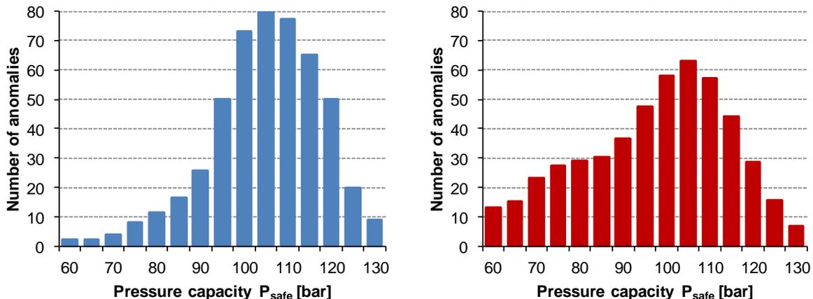
Figure 5: Two histograms of anomaly pressure capacity with same minimum  $P_{safe}$  (60 bar): left: few anomalies with low  $P_{safe}$ ; right: many anomalies with low  $P_{safe}$
