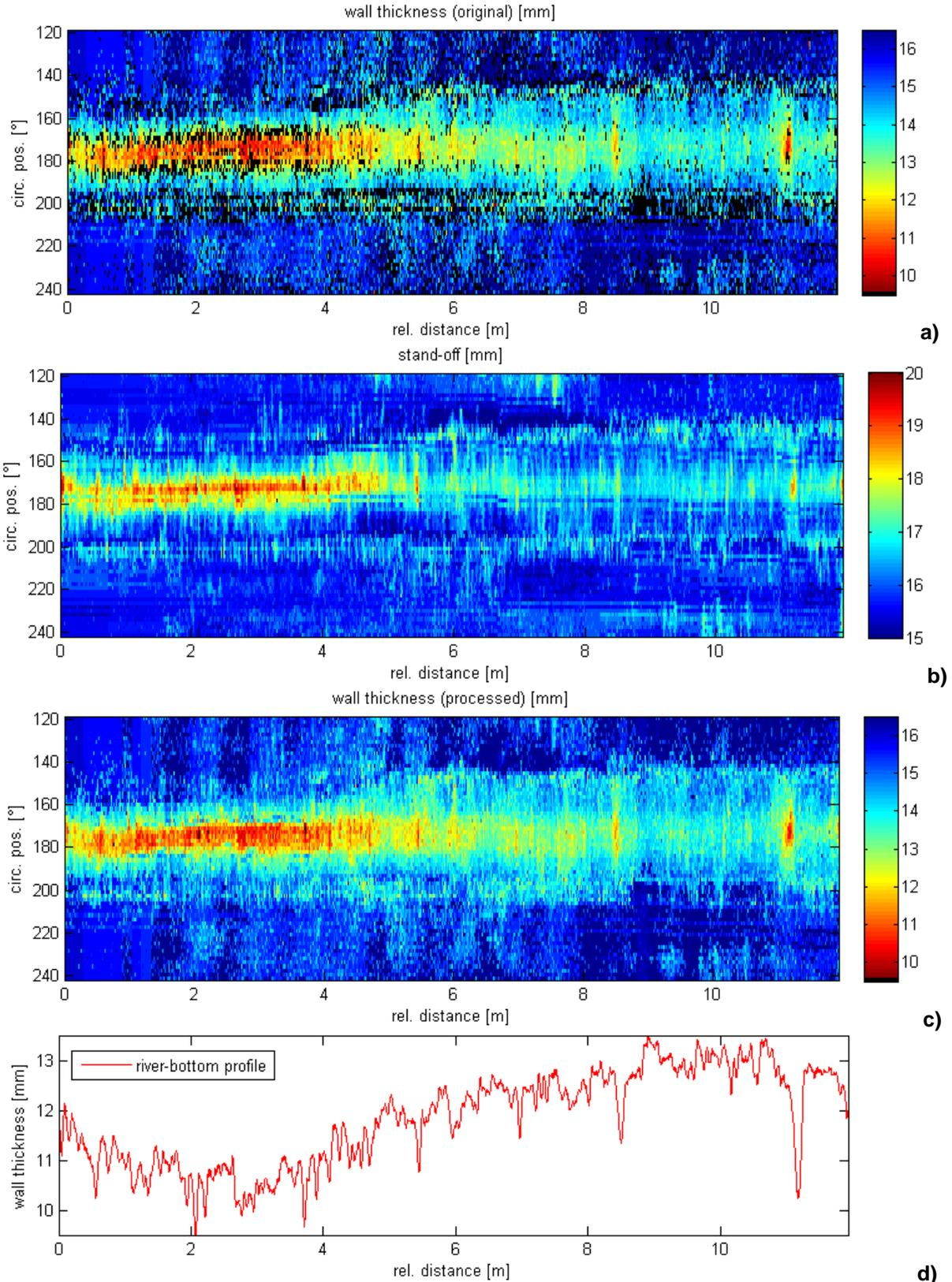
**Figure 7: Filtering of WT data as basis for construction of RBPs: a) original WT data, b) stand-off data, c) filtered WT data, d) RBP extracted from filtered WT**
