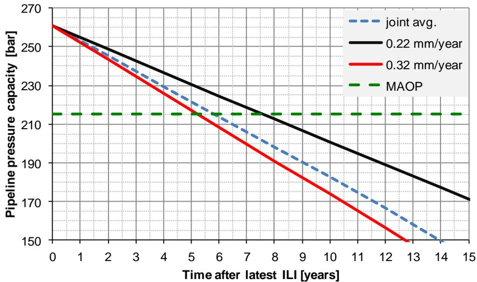
Figure 12: Extrapolation of pipeline safe working pressure
