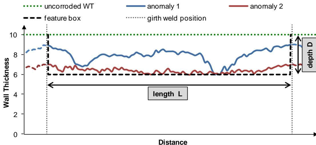
Figure 4: Sketch of two anomalies with same maximum depth and length but significantly different remaining wall thickness profiles.
