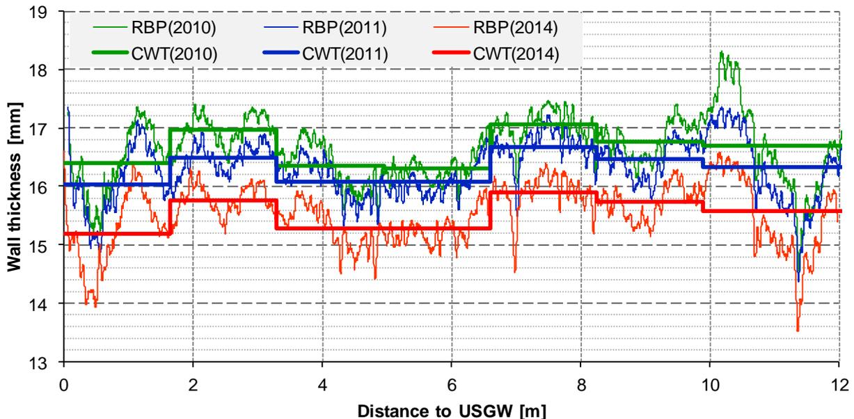
**Figure 9: RBPs of three consecutive ILIs and associated CWT profiles for one pipe joint**
