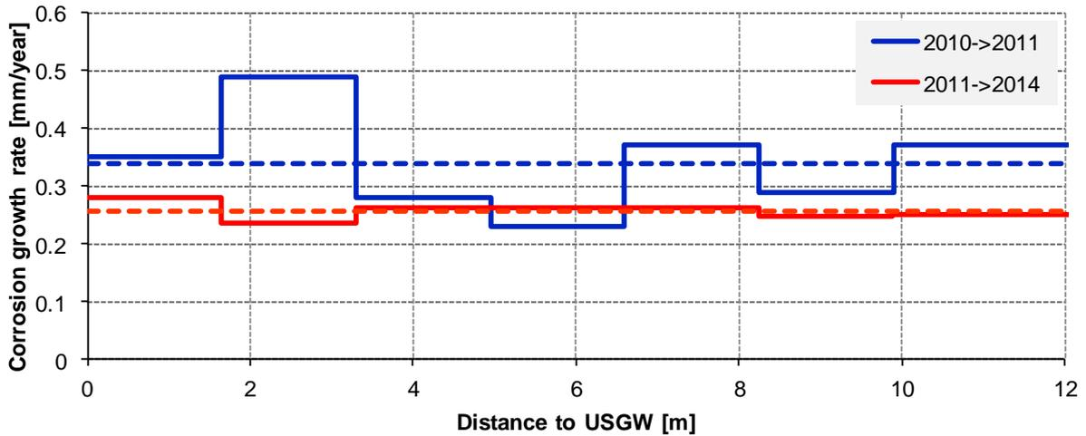
Figure 10: Corrosion growth rates calculated from CWT profiles of Figure 9
