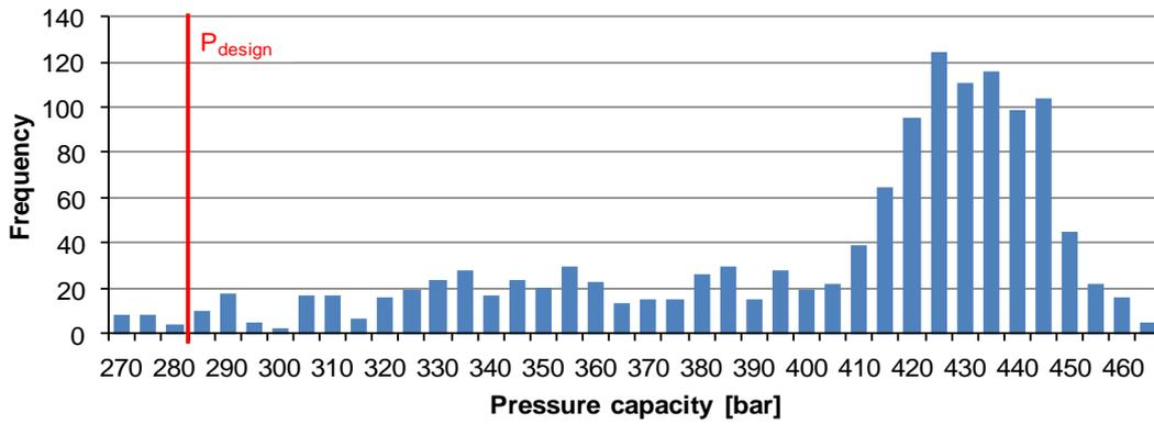
**Figure 8: Histogram of pressure capacity for pipe sections of 1.6m length**
