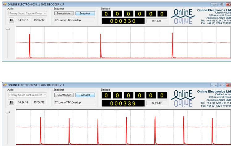
**Two Audioscope displays showing the background ping rate (top) and confirmation of pig passage (bottom). Note: the difference in the ping rate is clearly observable and simple to interpret**
