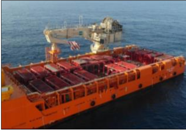
Figure 6: Nitrogen Dewatering Spread
