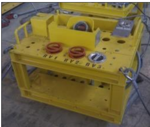
Figure 4: Remote Hydrotest Data-Logging Skid
