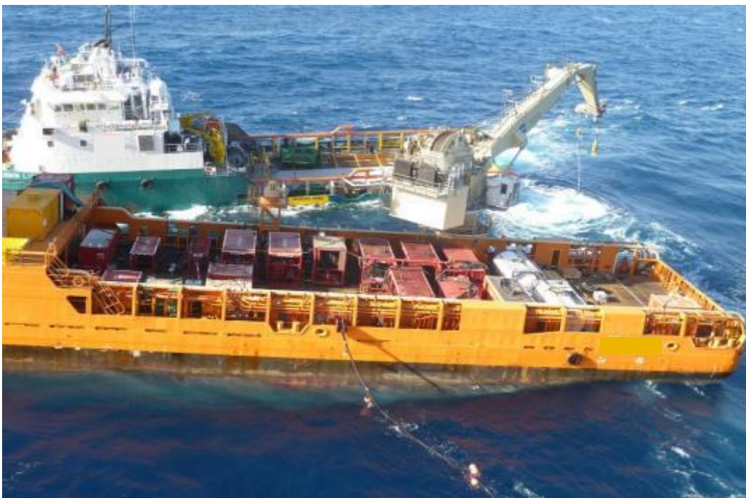
Figure 12: Vessel crane performing subsea PLT/ILI delivery
