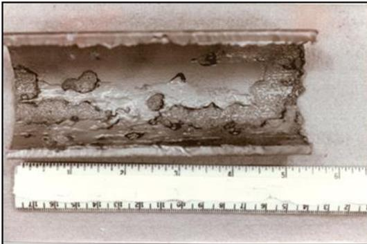
Example of CO<sub>2</sub> corrosion on a riser
