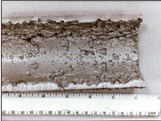
Example of CO<sub>2</sub> corrosion caused by condensation
