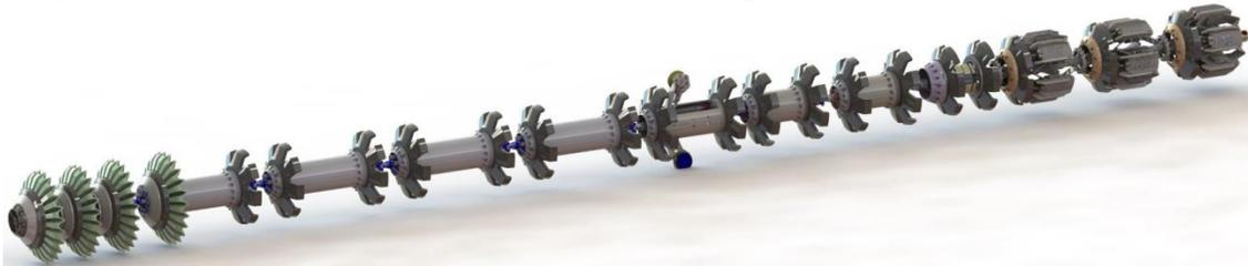
**Figure 11: Dual Diameter tool for high-resolution wall thickness measurement, 275 bar capable**
