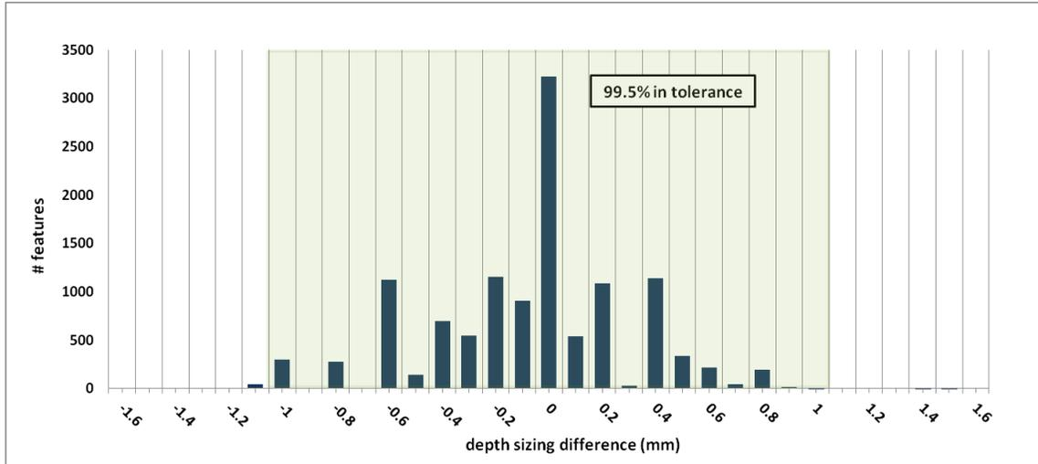
**Figure 9: Histogram of depth sizing deviation for one of the test runs. In total 99.5% of flaws are within specified depth sizing accuracy.**
