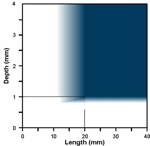
**Figure 6: Definition for crack and crack-like anomaly classification based on length and depth. Colored area shows application range of EVO Series 1.0 UC technology for detection and sizing of crack and crack-like anomalies.**
