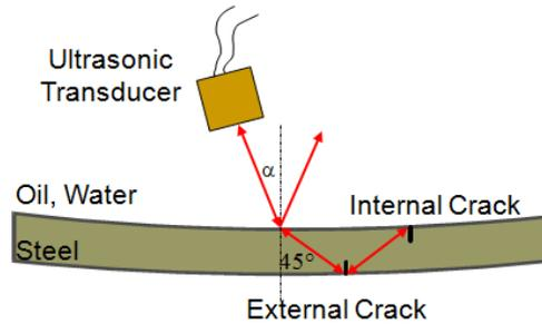
**Figure 2: Sketch for UT crack detection measurement principle**
