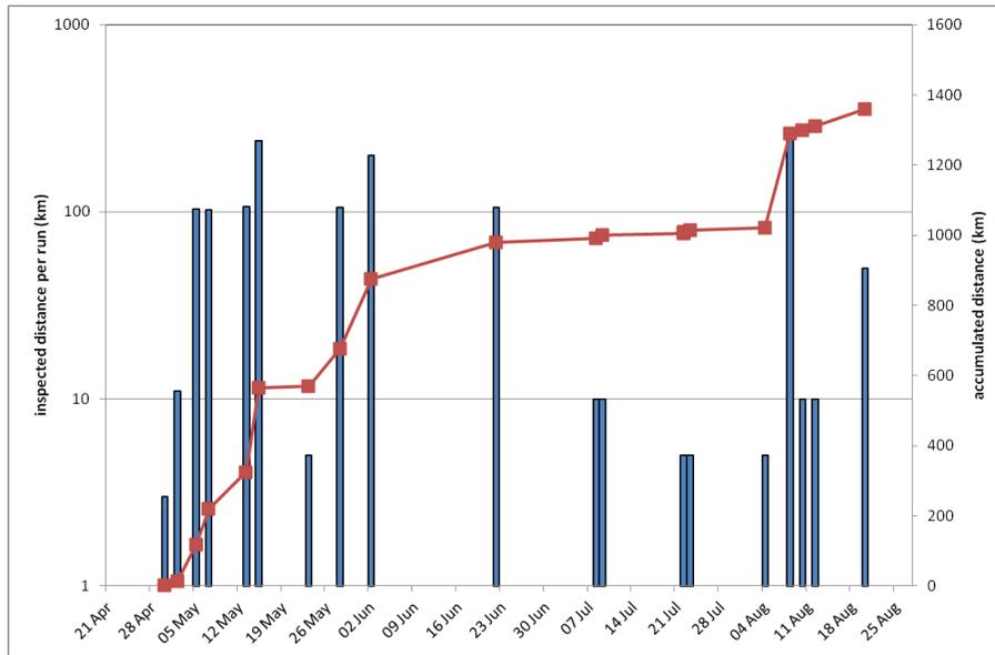
Figure 8: Utilization of 12" test loop over time. Individual run distance (blue) and accumulated distance in km is shown.
