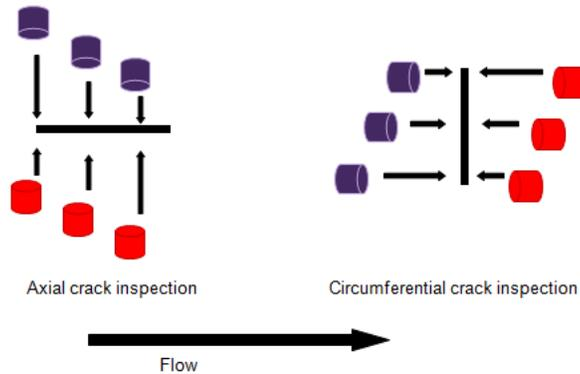
**Figure 3: Schematic drawing illustrating axial (left) and circumferential (right) transducer arrangement**
