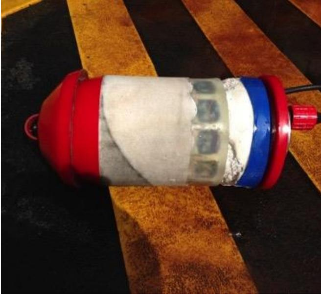
**Figure 6: Sensor array in a circular belt design.**
