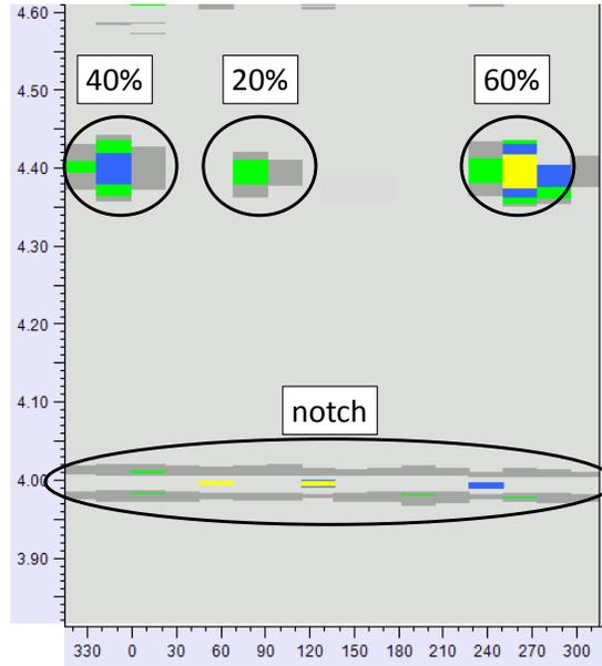
**Figure 13: Erosion type defects (type B) in the top of the figure.**
