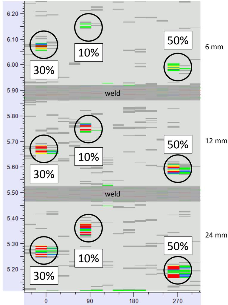
**Figure 14: Signals of metal loss defects underneath the liner.**
