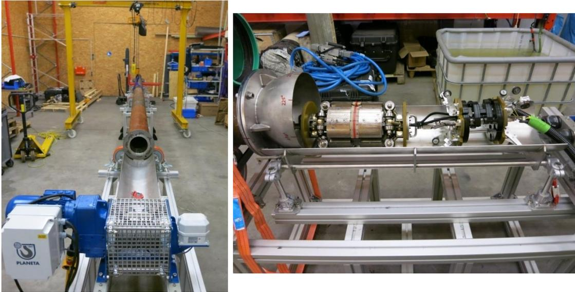
**Figure 9: Left: Set-up of the test spool, Right: Prototype inspection device**
