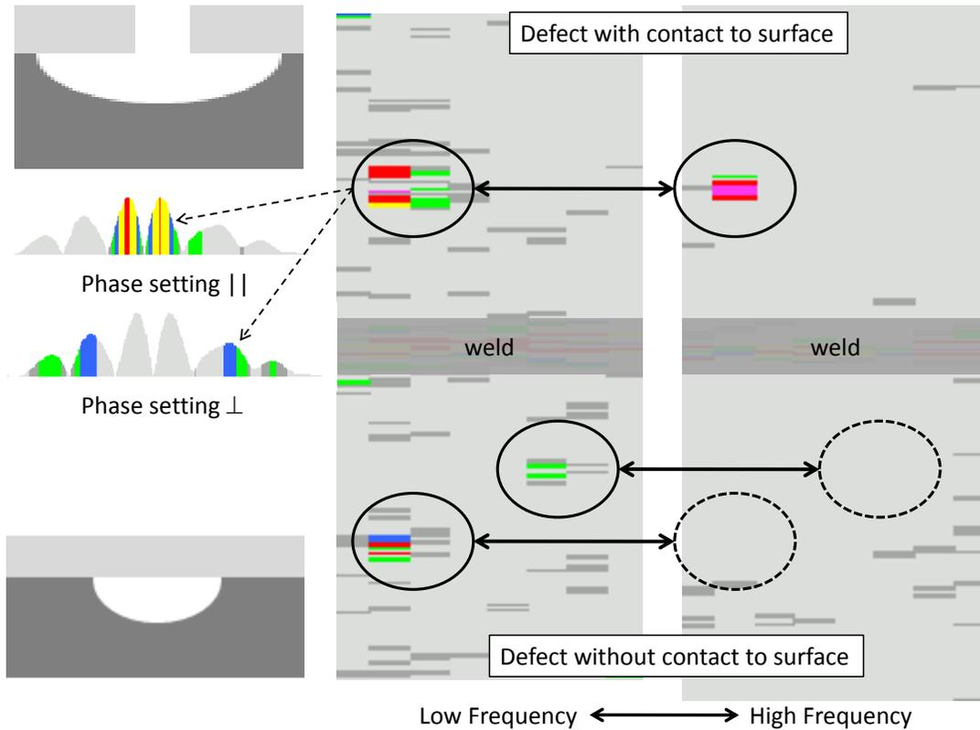
**Figure 15: Comparison of internal metal loss defects at different frequencies (center to right). The defect with contact to the surface remains visible even at higher frequencies (top). The defect hidden under the liner disappears (bottom).**
