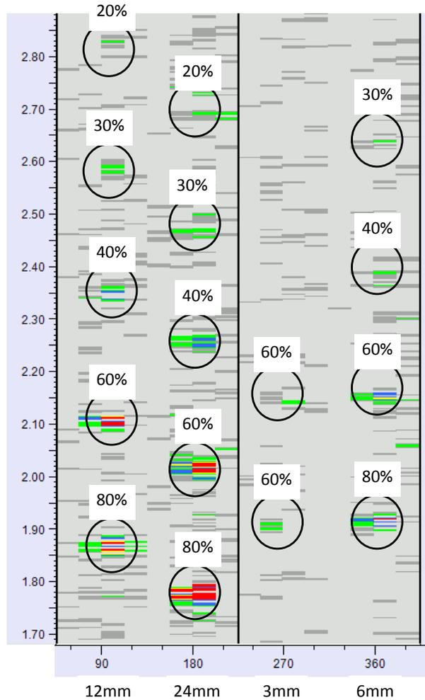
**Figure 10: Data screen shot of external defects**
