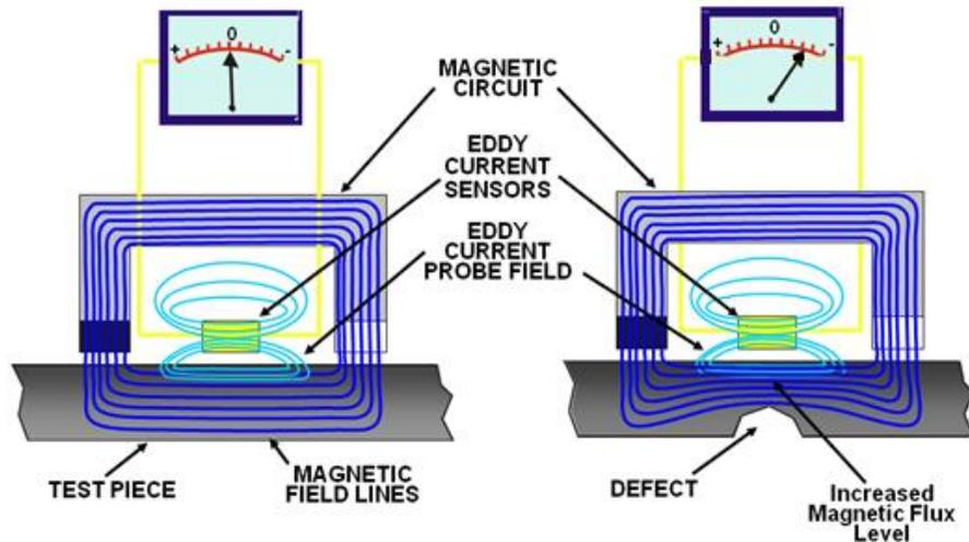
Figure 1: Principle of the MEC™ technology (Magnetic Eddy Current) also known as a further developed technique from Saturation Low Frequency Eddy Current (SLOFEC™).
