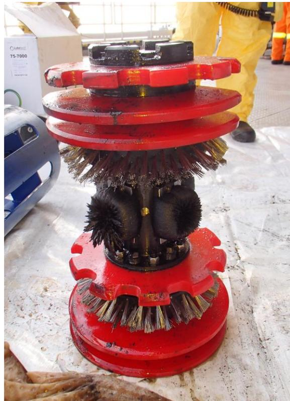
Figure 3: Brush pig with debris
