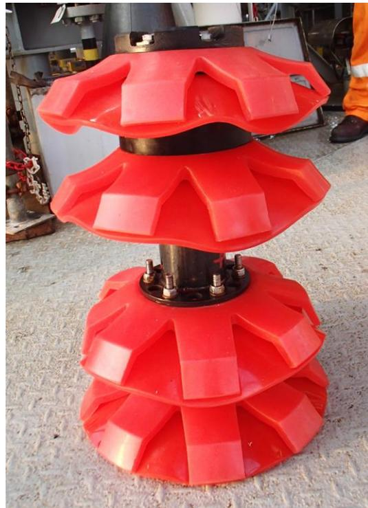
Figure 2: De-sanding pig
