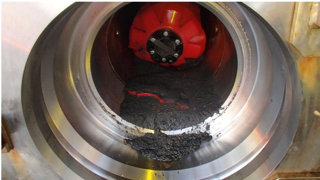
**Figure 4: De-sanding pig and debris in receiver during operational cleaning**
