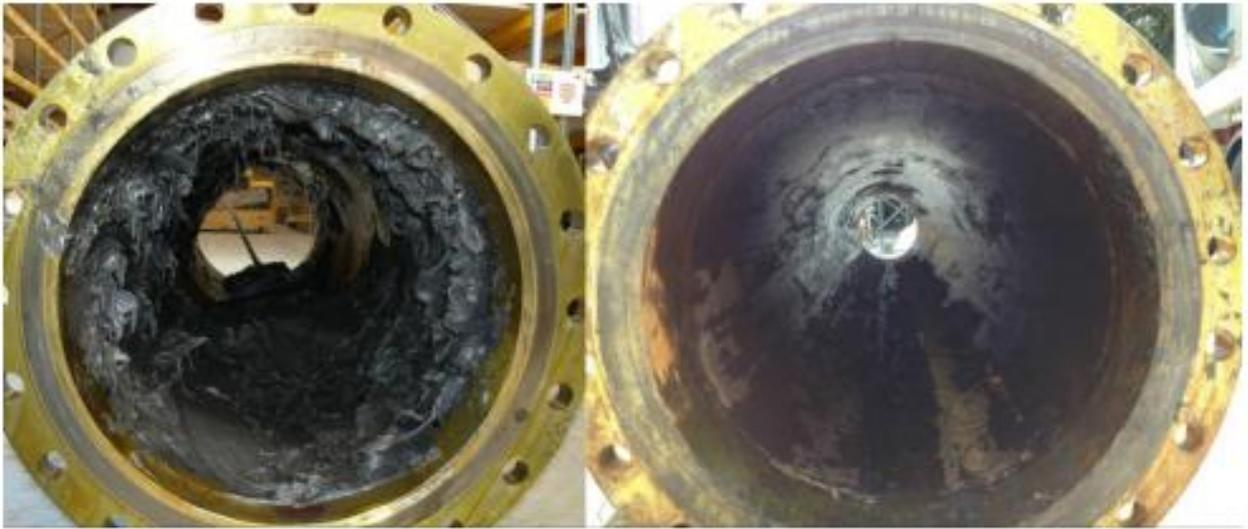
Figure 4 A 3m portion of the 24" pipe was loaded with 250 kgs of sand in one test, and 100 kgs of dyed petroleum wax in another, ice pigging cleaned both contaminants very effectively.
