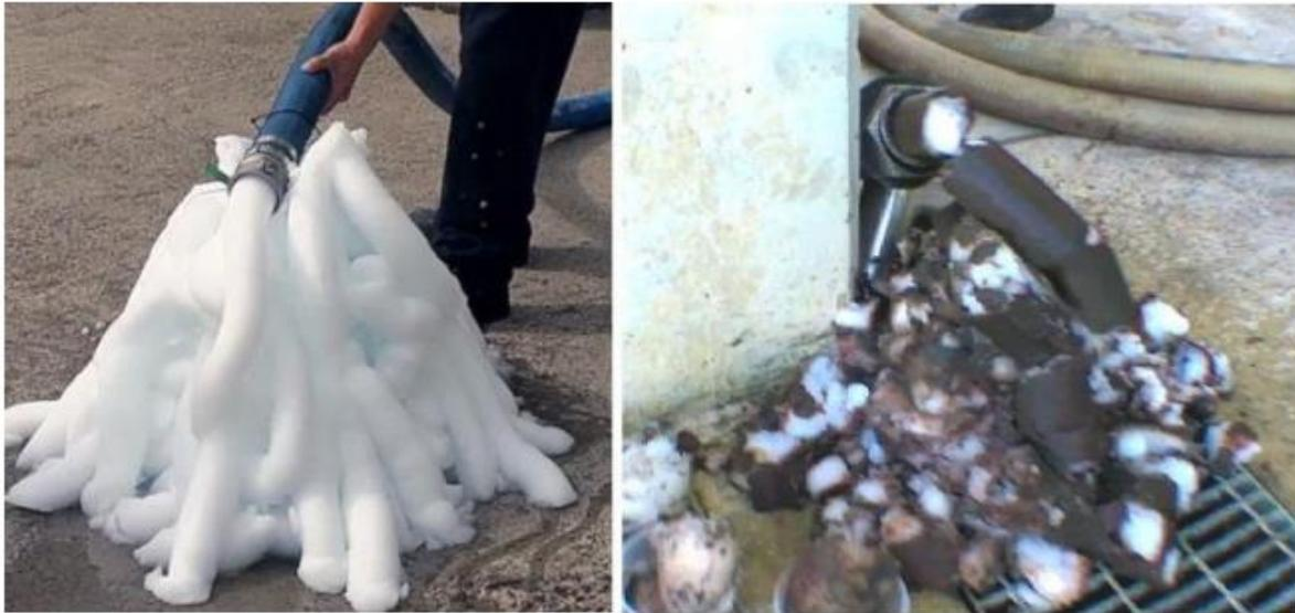
Figure 1 The ice slurry used in ice pigging is very thick and dry, whilst still flowable. It cleans tough deposits by abrasion.
