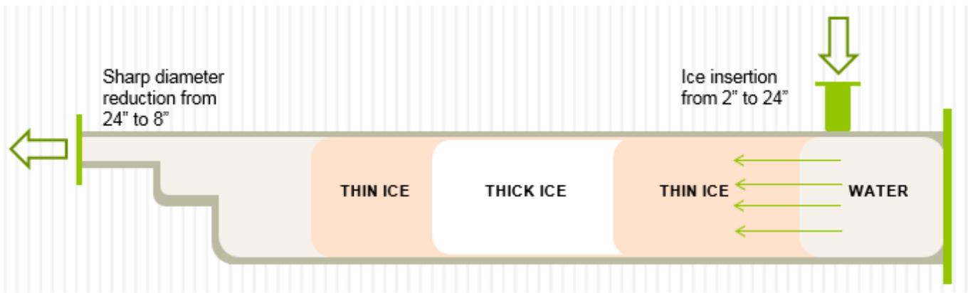
Figure 6, diagram showing how the ice slurry was injected to account for length to diameter ratio of the test rig.
