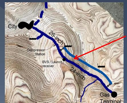
Model the process and pigging of a complex gas network
