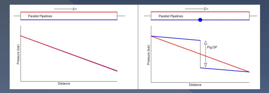
Two lines with common inlet and outlet. Flow is proportional to pressure gradient. Pressure gradient less in line with pig so risk of stalling as flow diverts
