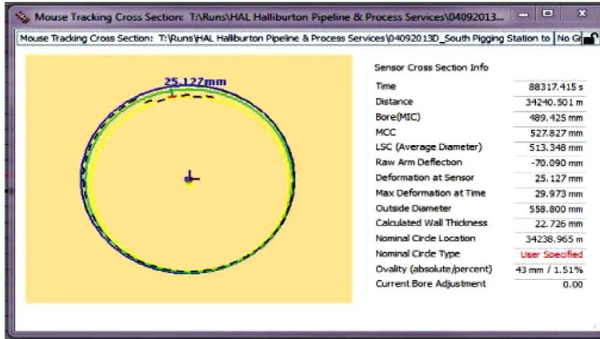
Figure 2—Data received from caliper survey of anomaly on Segment C
