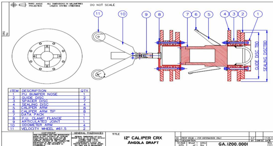
Figure 5—Segment W 12-in. caliper pig
