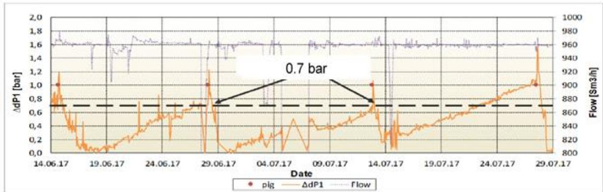
Figure 8. The graph shows 0.7 bar pressure build up between two pig launches.
