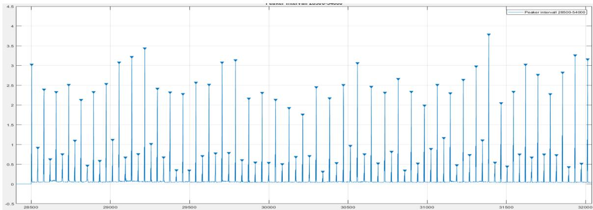
Figure 2. Girth weld pass identification by MATLAB filter.
