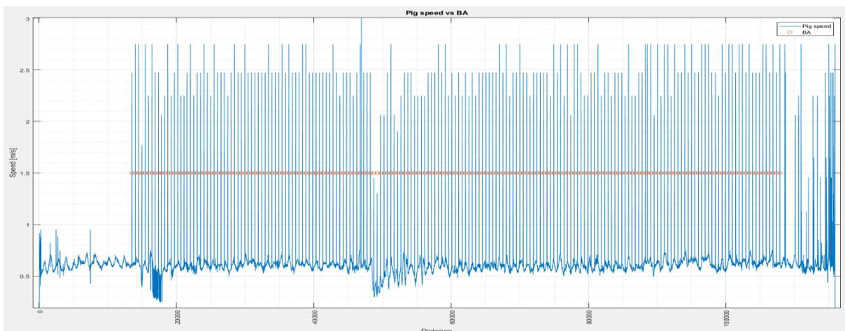
Figure 3. Joint speed plot with peaks for buckle arrestors and location of buckle arrestors.
