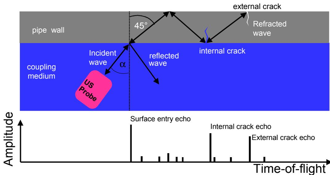
**Figure 4: The principle arrangement for ultrasonic crack detection. Sound waves will travel through the pipe wall at an angle close to 45 °.**
