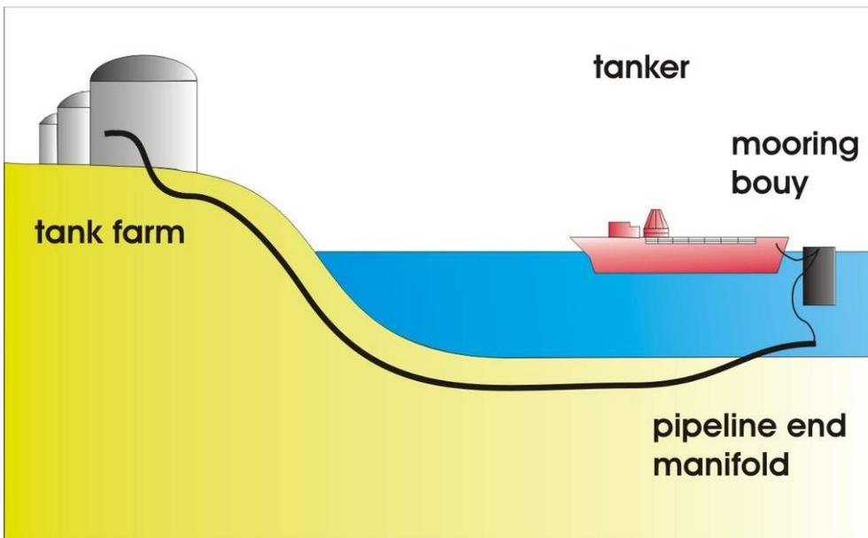
Fig. 4: (Case history no. 3) Schematics of the tanker unloading facilities
