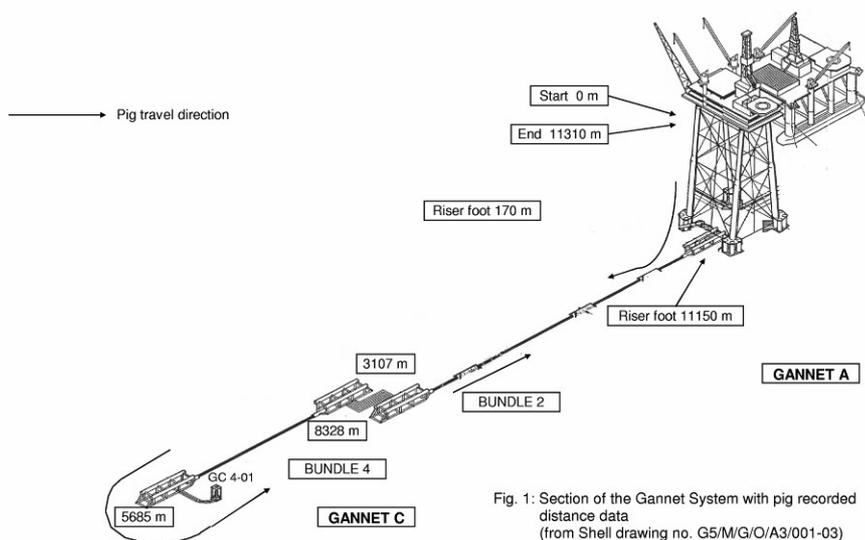
Fig. 1: Section of the Gannet System with pig recorded distance data (from Shell drawing no. G5/M/G/O/A3/001-03)
